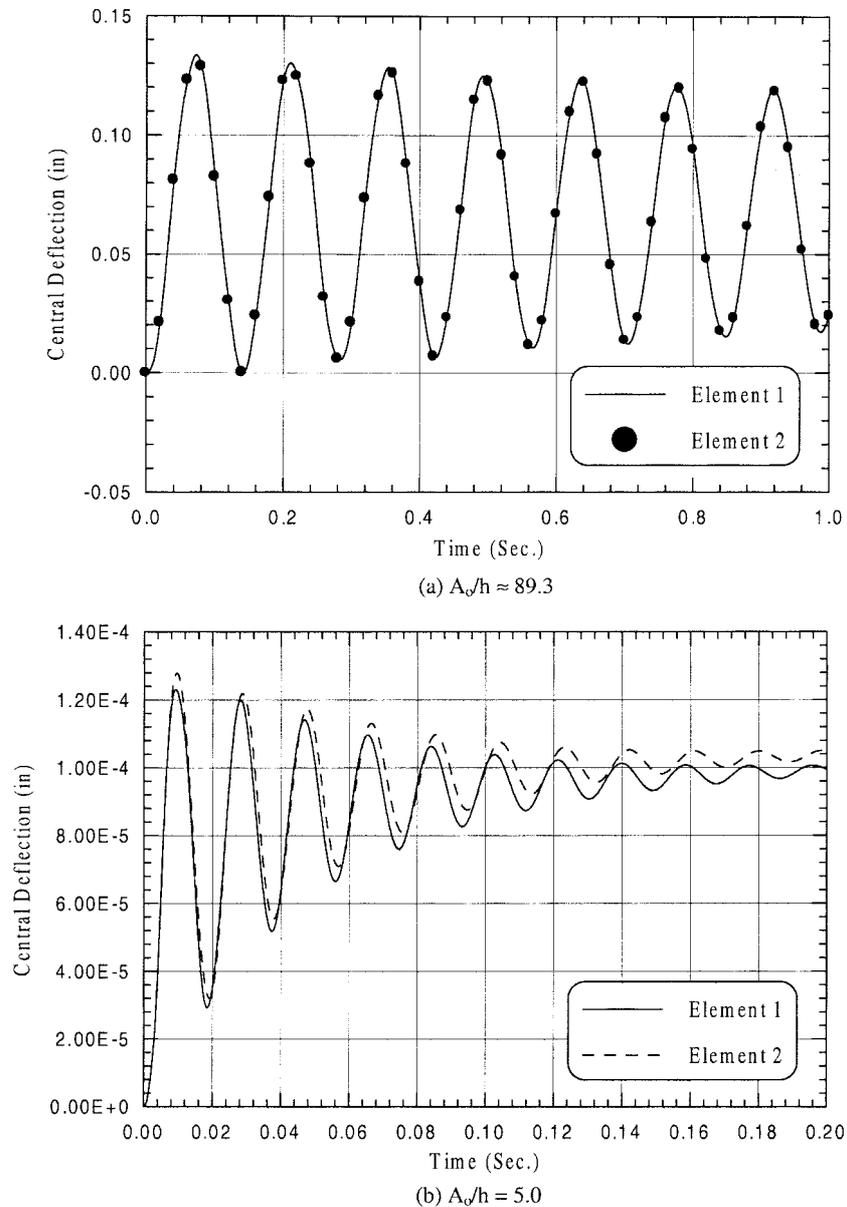
Fig. 1 The viscoelastic deflection of a simply supported plate with  $(0^\circ_{10}/90^\circ_{10})_s$ -stacking sequence
