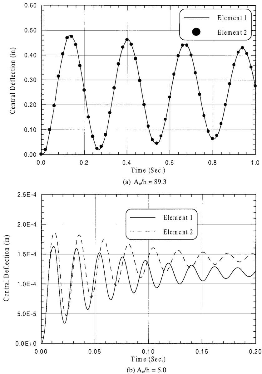
Fig. 2 The viscoelastic deflection of a simply supported unsymmetric Laminate with  $(0^{\circ}_{20}/90^{\circ}_{20})_t$  -lamination scheme
