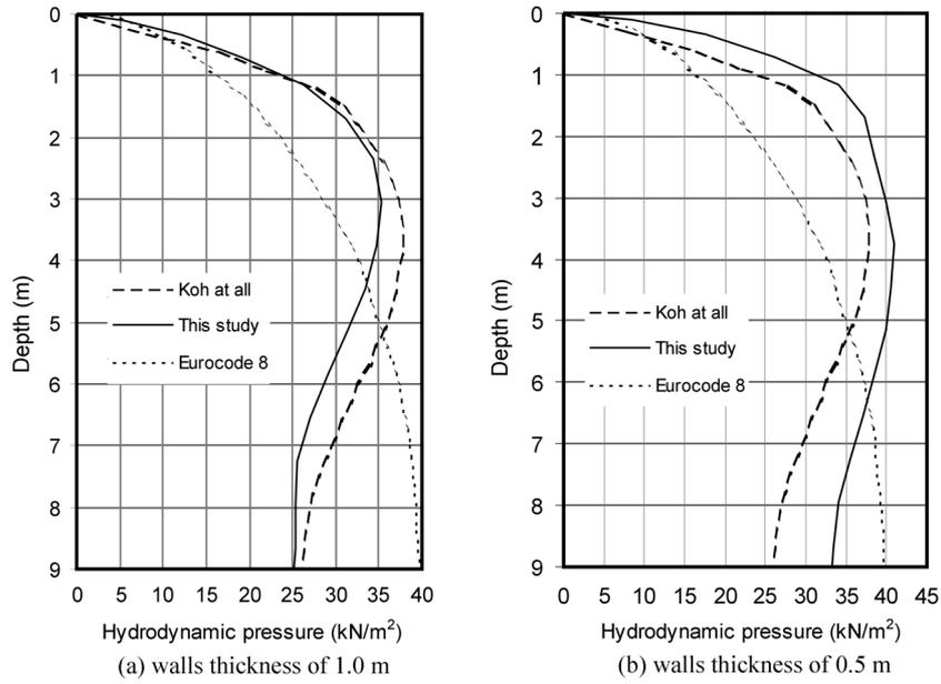
Fig. 8 Hydrodynamic pressure distribution obtained from assuming walls are flexible
