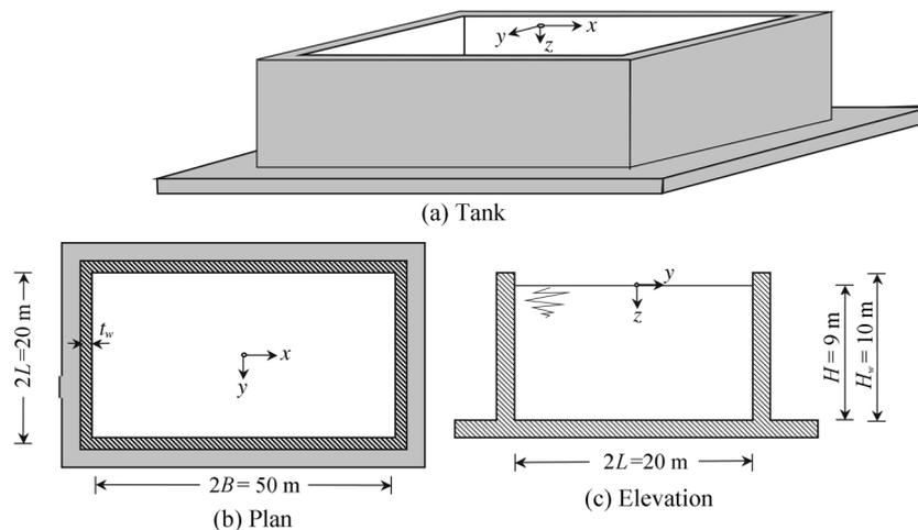
Fig. 4 Plan and elevation of the sample rectangular tank
