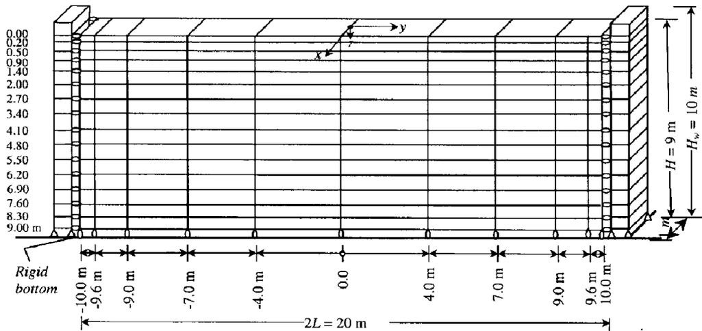
Fig. 7 Finite element mesh considered for unit width of flexible solution
