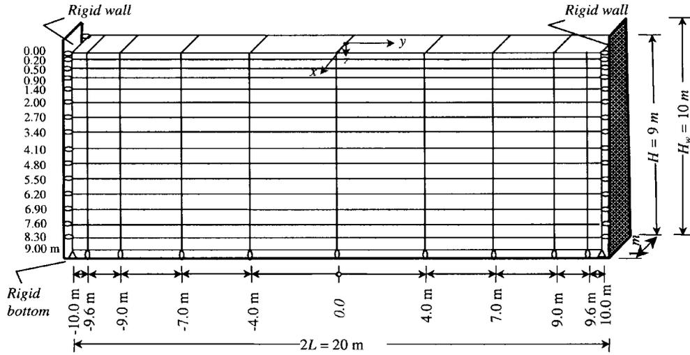
Fig. 5 Finite element mesh considered for unit width of tank in rigid solution
