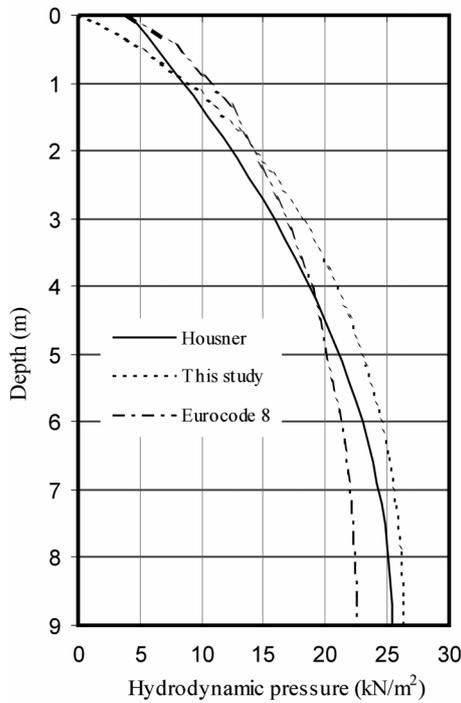
Fig. 6 Hydrodynamic pressure distributions obtained from assuming walls are rigid
