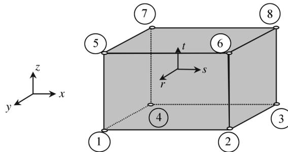
Fig. 1 Fluid finite element considered
