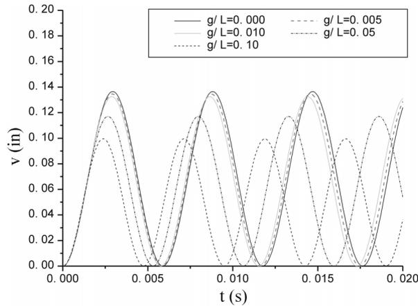
Fig. 3 Free end deflection of gradient elastic cantilever beam versus time for various values of  $g/L$
