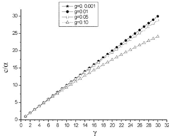
Fig. 2 Dispersion curves (phase velocity-wavenumber relation) for various values of  $g$
