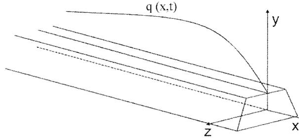
Fig. 1 Geometry and loading of a straight prismatic beam
