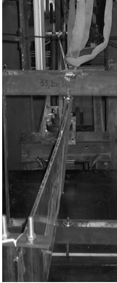
Fig. 13 Buckling of large specimen
