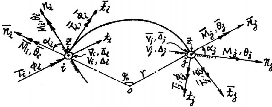
Fig. 1 Coordinate system and end forces, displacements notations
