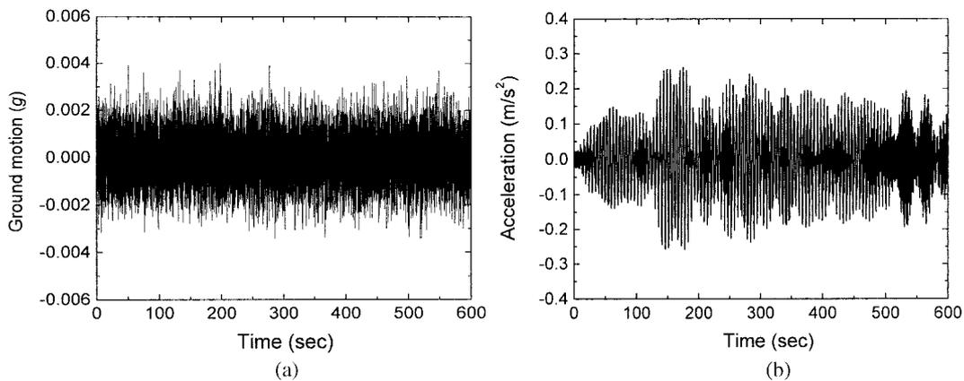
Fig. 14 Ground motion and acceleration response time histories: (a) Ground motion, (b) Acceleration response at the top of appendage
