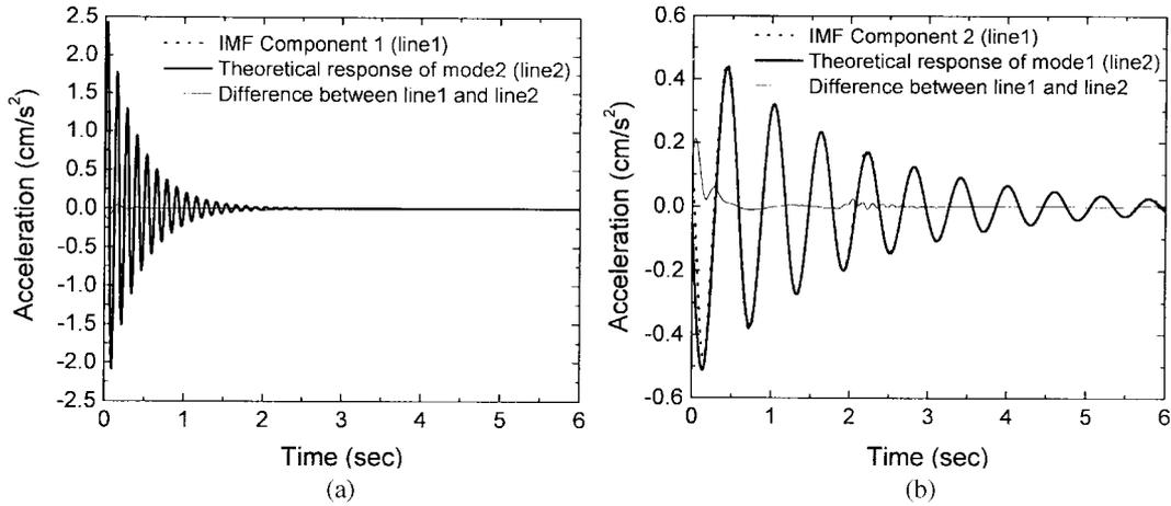
Fig. 4 The IMF components and the modal responses (well-separated modes): (a) The first IMF component and the second modal response, (b) The second IMF component and the first modal response
