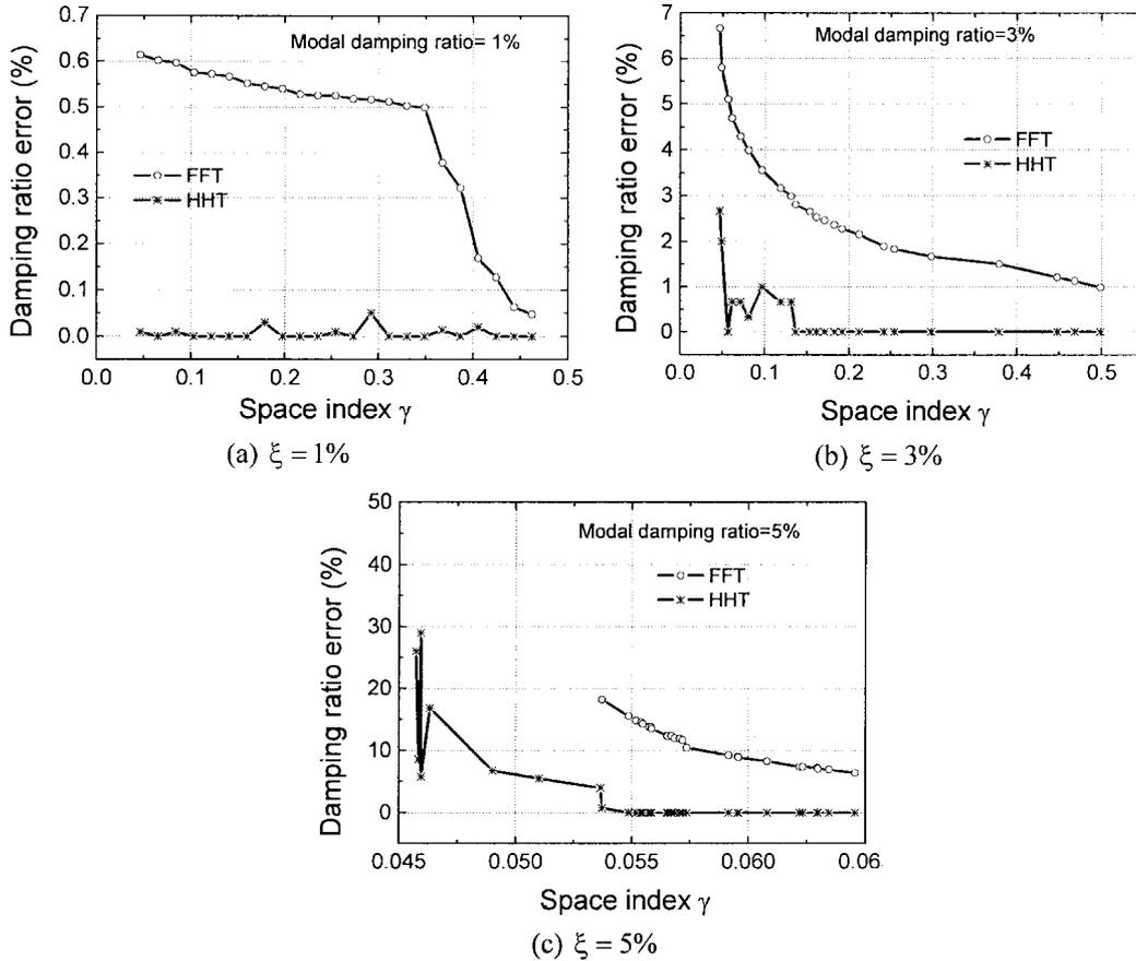
Fig. 12 Variation of damping ratio error with space index; (a)  $\xi = 1\%$ , (b)  $\xi = 3\%$ , (c)  $\xi = 5\%$
