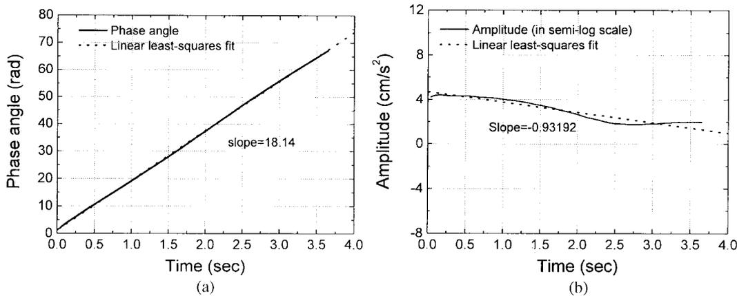
Fig. 9 Instantaneous functions of the first IMF component (closely spaced modes): (a) Phase angle and linear least-squares fit, (b) Amplitude and linear least-squares fit
