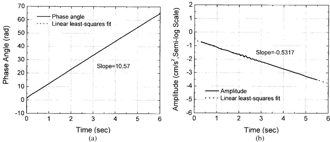
Fig. 5 Instantaneous functions of the first IMF component (well-separated modes): (a) Phase angle and linear least-squares fit, (b) Amplitude and linear least-squares fit
