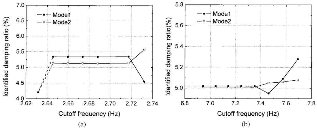
Fig. 11 Sensitivity of the modal damping ratio identification to the cutoff frequency: (a) 2DOF system with closely spaced modes of vibration, (b) 2DOF system with well-separated modes of vibration
