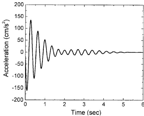
Fig. 6 Acceleration time history for closely spaced modes of vibration
