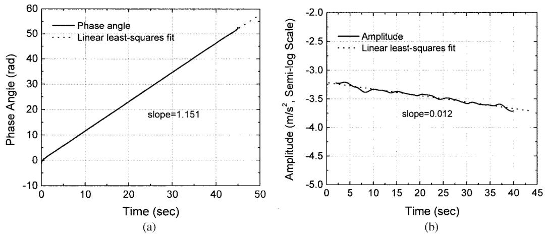
Fig. 17 Instantaneous functions of the first free modal response (shear building): (a) Phase angle and linear least-squares fit, (b) Amplitude and linear least-squares fit
