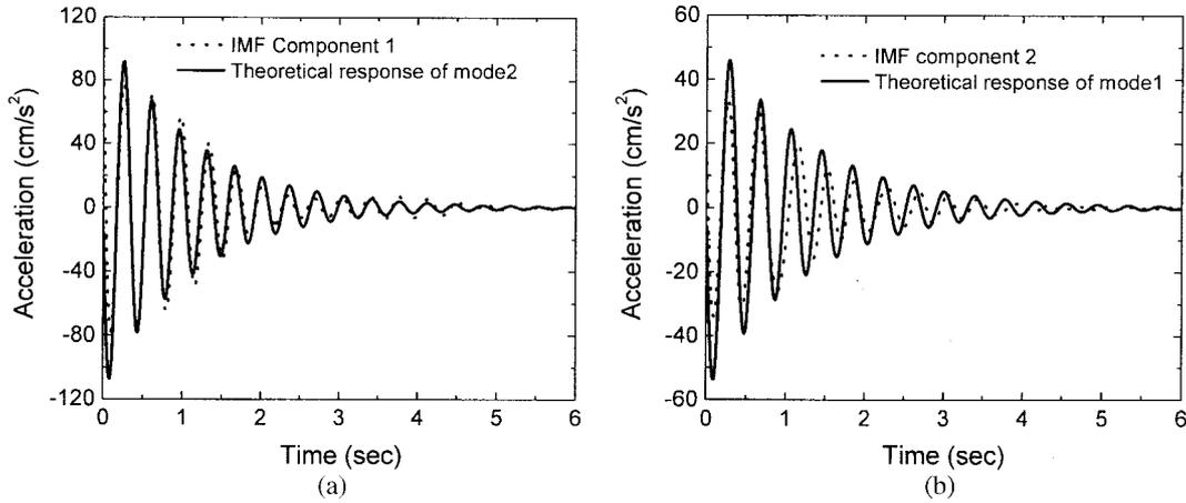
Fig. 8 The IMF components and the modal responses (closely spaced modes): (a) The first IMF component and the second modal response, (b) The second IMF component and the first modal response
