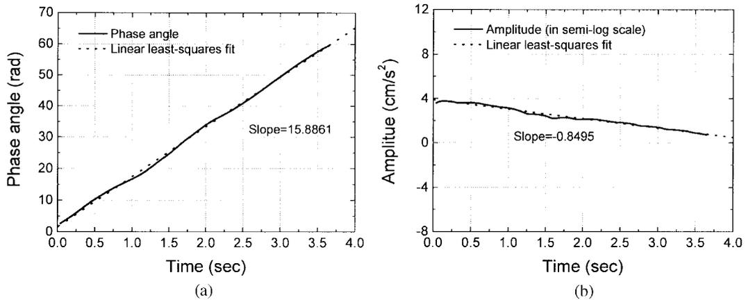
Fig. 10 Instantaneous functions of the second IMF component (closely spaced modes): (a) Phase angle and linear least-squares fit, (b) Amplitude and linear least-squares fit
