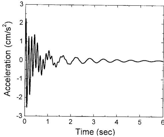
Fig. 2 Acceleration time history for well-separated modes of vibration
