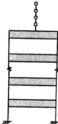
Fig. 13 Shear building with light appendage
