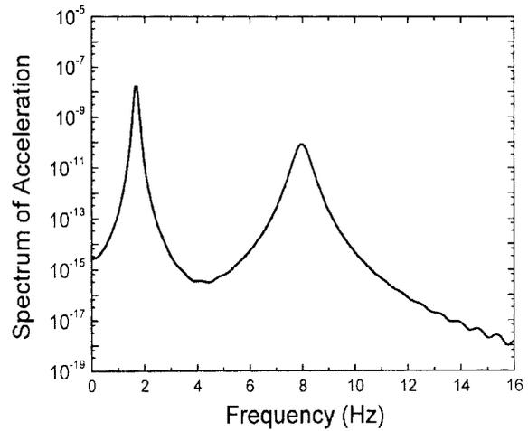
Fig. 3 Power spectrum for the time history shown in Fig. 2
