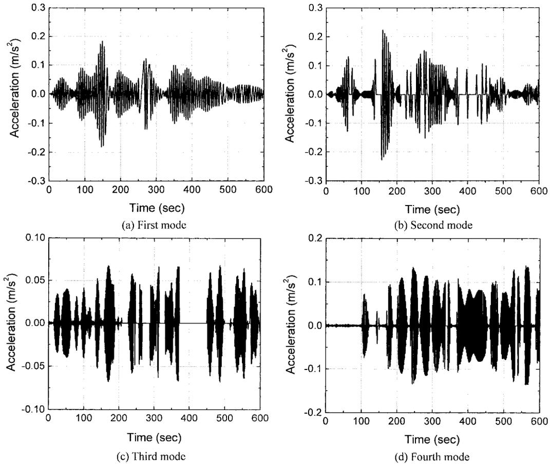
Fig. 16 The first four total modal responses: (a) First mode, (b) Second mode, (c) Third mode, (d) Fourth mode
