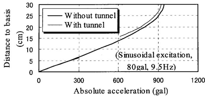
Fig. 8 Vibrational mode of accelerations in central ground (based on dynamic analysis)
