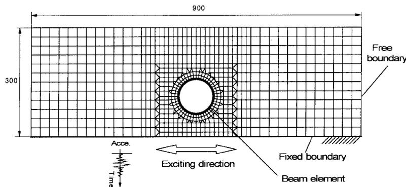
Fig. 3 The finite element idealization of ground-tunnel composite in dynamic numerical model
