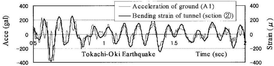
Fig. 12 Comparison between wavelines of ground acceleration and wavelines of tunnel strain
