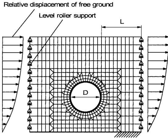
Fig. 4 Static analysis using ground-tunnel composite finite element model
