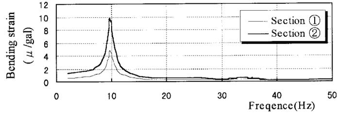
Fig. 10 Resonance curves of bending strains of the tunnel (based on tests)
