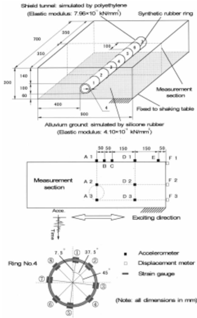
Fig. 1 Details of test model and measurement points
