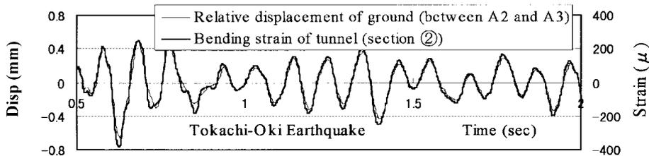
Fig. 13 Comparison between wavelines of ground displacement and wavelines of tunnel strain
