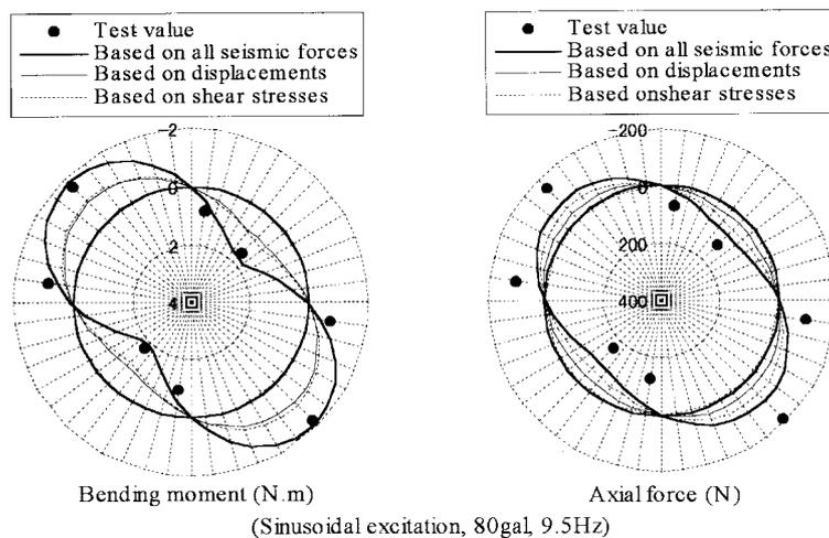
Fig. 19 Test and analytical results of maximum sectional forces of the tunnel (beam-spring model)
