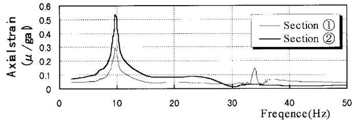
Fig. 11 Resonance curves of axial strains of the tunnel (based on tests)
