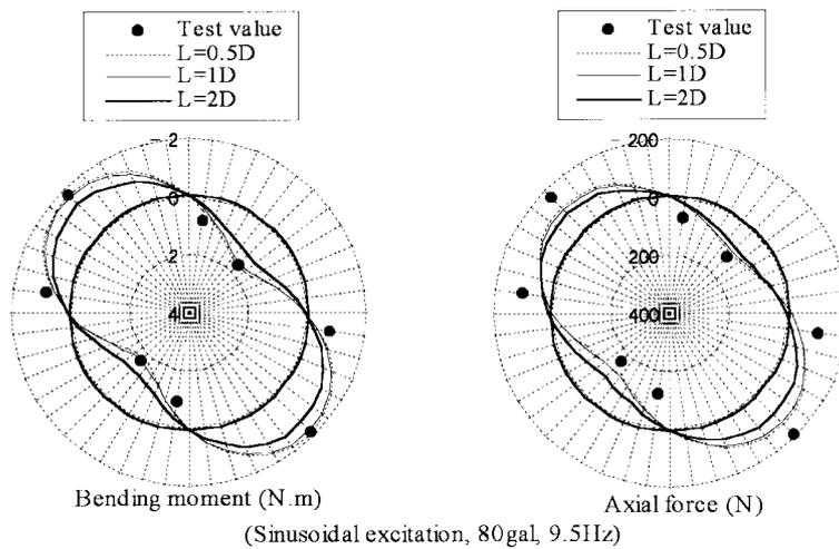
Fig. 17 Test and analytical results of maximum sectional forces of the tunnel (static FE model)
