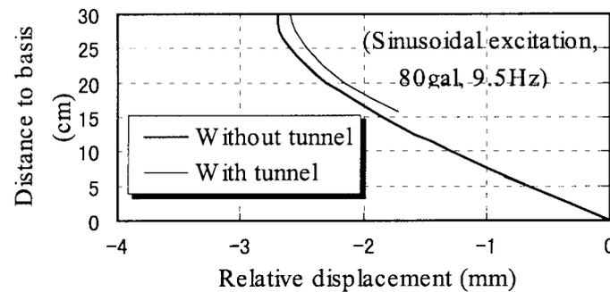
Fig. 9 Vibrational mode of relative displacements in central ground (based on dynamic analysis)
