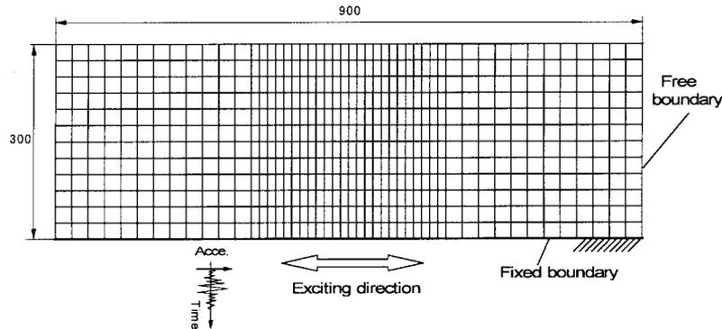
Fig. 2 The finite element idealization of free ground in dynamic numerical model
