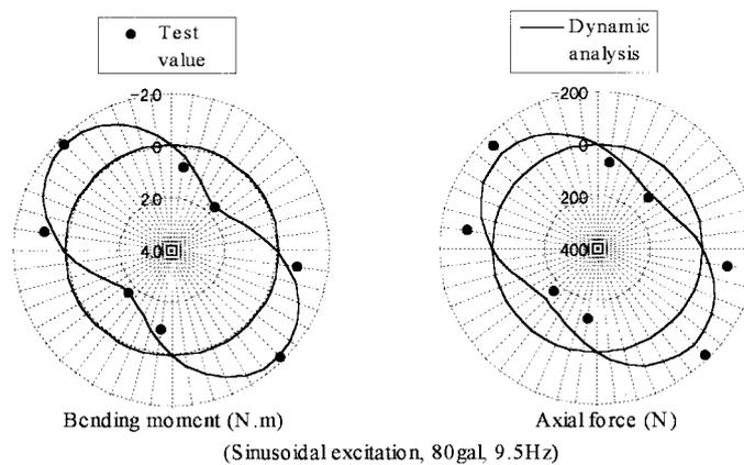
Fig. 14 Test and dynamic analytical results of maximum sectional forces of the tunnel
