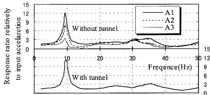
Fig. 6 Resonance curves of ground accelerations (based on tests)
