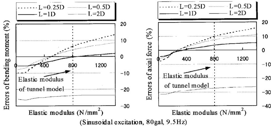
Fig. 18 Errors of sectional forces based on static FE model relatively to the dynamic analysis
