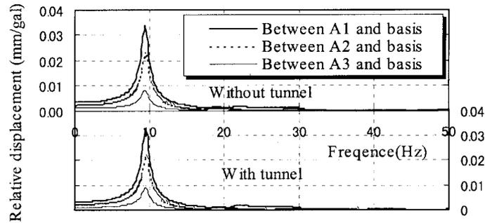
Fig. 7 Resonance curves of ground relative displacements (based on dynamic analysis)
