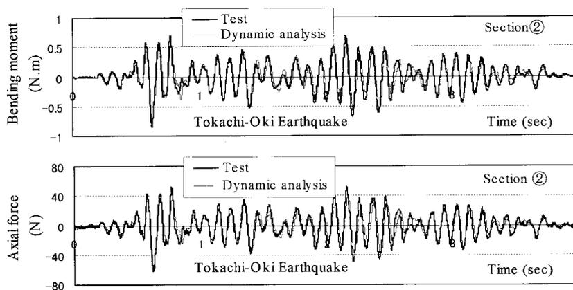
Fig. 15 Test and analytical results of sectional forces of the tunnel
