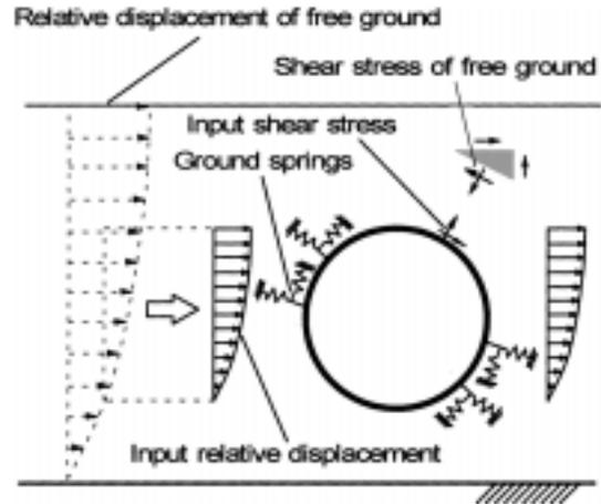
Fig. 5 Static analysis using beam-spring element model
