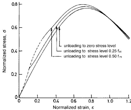
Fig. 5 Common point curves normal to bed joint
