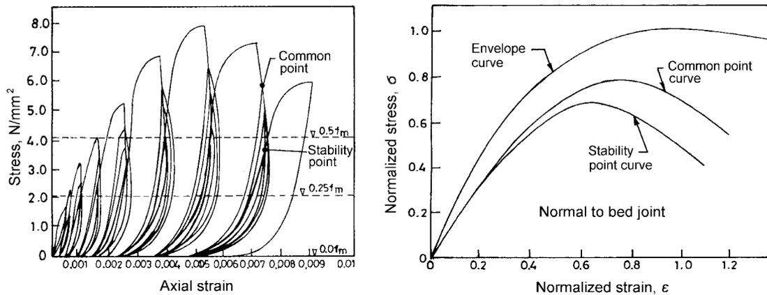
Fig. 2 (a) Typical stress-strain hysteresis for full unloading-reloading, (b) Typical analytical stress-strain curves for full unloading-reloading
