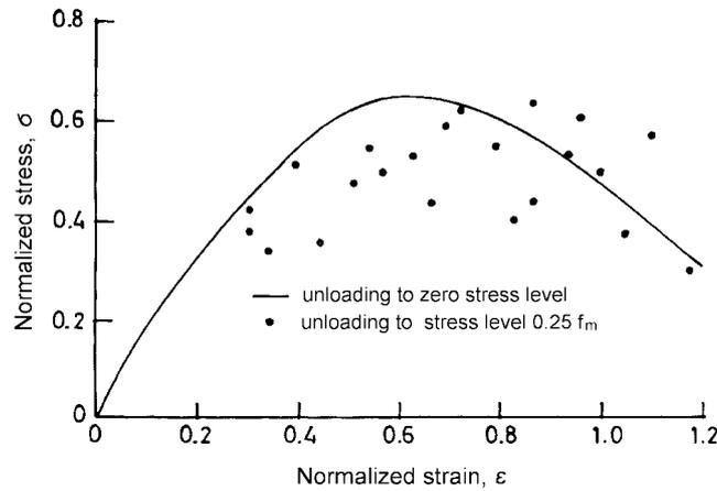
Fig. 7 Stability point curves normal to bed joint
