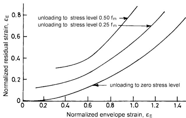
Fig. 10 Variation of residual strain with envelope strain parallel to bed joint
