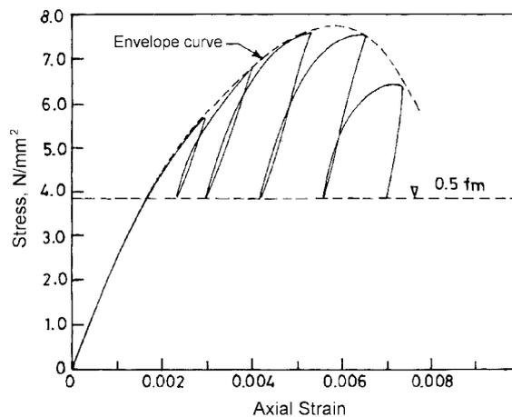
Fig. 4 Common point test for partial unloading: Parallel to bed joint
