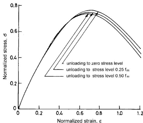
Fig. 6 Common point curves parallel to bed joint
