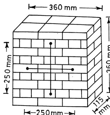
Fig. 1 Specimen dimension and LVDTs arrangement
