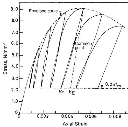
Fig. 3 Common point test for partial unloading: Normal to bed joint
