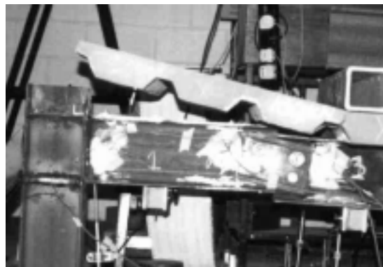
Fig. 14 The separation of the slab (Beam 1)
