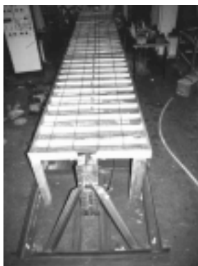
Fig. 9 Test specimen before casting concrete
