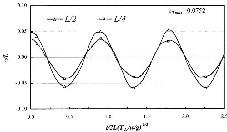
Fig. 10 Vibration amplitude of  $v$  at mid span and quarter span for  $S=800$  m and  $E=2.294 \times 10^6$  kN/m<sup>2</sup>
