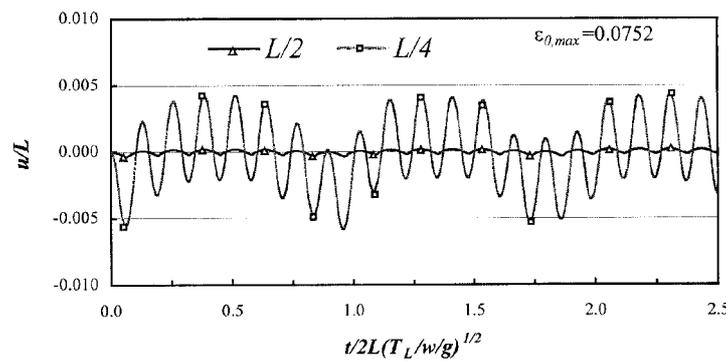
Fig. 11 Vibration amplitude of  $u$  at mid span and quarter span for  $S=800$  m and  $E=2.294 \times 10^6$  kN/m<sup>2</sup>
