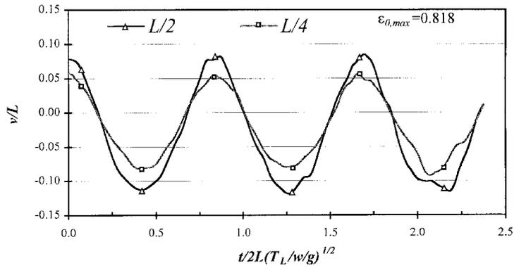
Fig. 13 Vibration amplitude of  $v$  at mid span and quarter span for  $T_L=17,000$  kN and  $E=1.794 \times 10^5$  kN/m<sup>2</sup>
