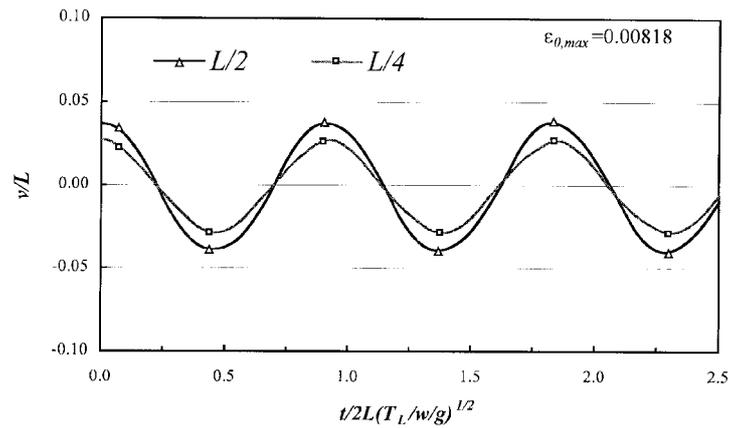
Fig. 17 Vibration amplitude of  $v$  at mid span and quarter span for  $T_L=17,000$  kN and  $E=1.794 \times 10^7$  kN/m<sup>2</sup>
