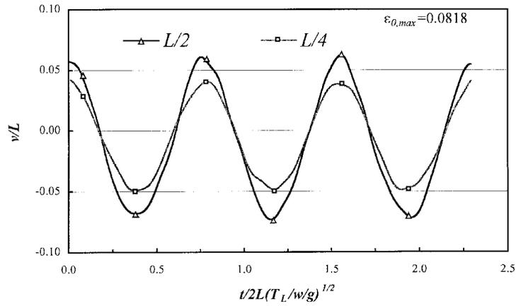
Fig. 15 Vibration amplitude of  $v$  at mid span and quarter span for  $T_L=17,000$  kN and  $E=1.794 \times 10^6$  kN/m<sup>2</sup>
