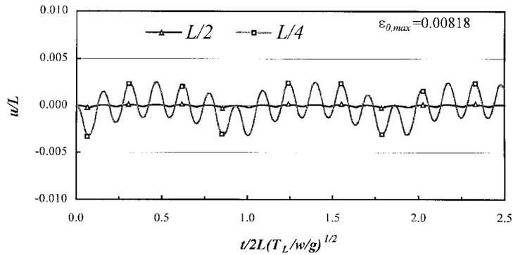
Fig. 18 Vibration amplitude of  $u$  at mid span and quarter span for  $T_L=17,000$  kN and  $E=1.794 \times 10^7$  kN/m<sup>2</sup>
