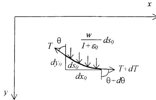
Fig. 2 Free body of infinitesimal cable segment
