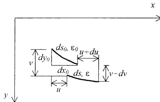
Fig. 3 Equilibrium and displaced positions of cable segment
