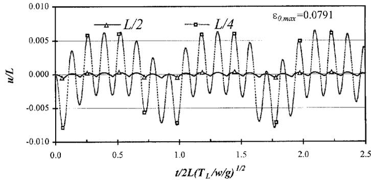
Fig. 9 Vibration amplitude of  $u$  at mid span and quarter span for  $S=800$  m and  $E=1.794 \times 10^6$  kN/m<sup>2</sup>
