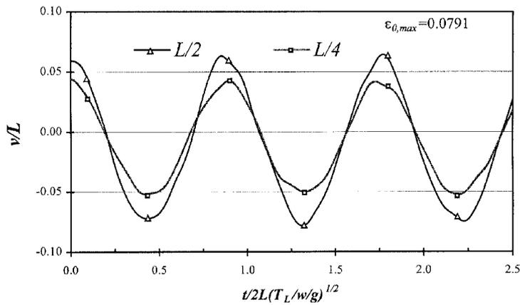
Fig. 8 Vibration amplitude of  $v$  at mid span and quarter span for  $S=800$  m and  $E=1.794 \times 10^6$  kN/m<sup>2</sup>
