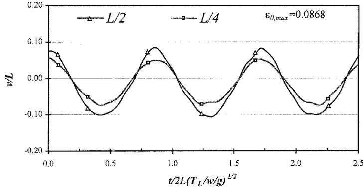
Fig. 6 Vibration amplitude of  $v$  at mid span and quarter span for  $S=800$  m and  $E=1.294 \times 10^6$  kN/m<sup>2</sup>
