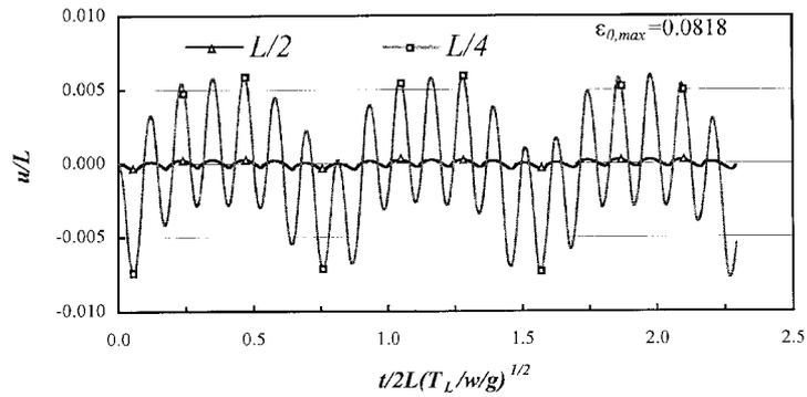
Fig. 16 Vibration amplitude of  $u$  at mid span and quarter span for  $T_L=17,000$  kN and  $E=1.794 \times 10^6$  kN/m<sup>2</sup>
