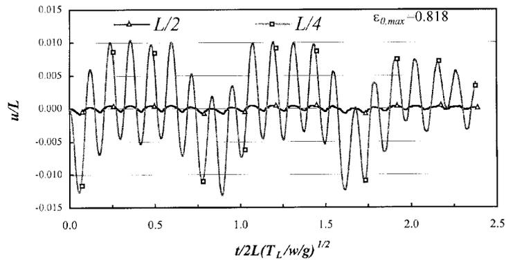
Fig. 14 Vibration amplitude of  $u$  at mid span and quarter span for  $T_L=17,000$  kN and  $E=1.794 \times 10^5$  kN/m<sup>2</sup>
