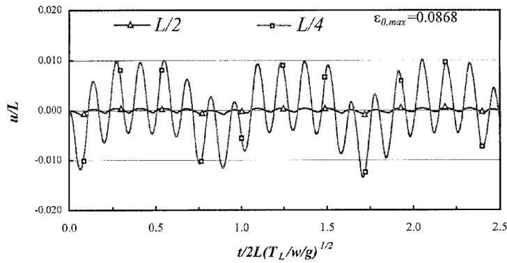
Fig. 7 Vibration amplitude of  $u$  at mid span and quarter span for  $S=800$  m and  $E=1.294 \times 10^6$  kN/m<sup>2</sup>
