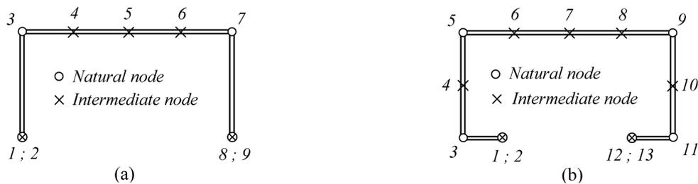
Fig. 2 (a) Plain and (b) lipped channel GBT cross-section discretisations
