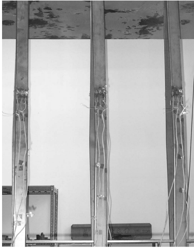
Fig. 7 Typical failure type of wall frames with channel bridging
