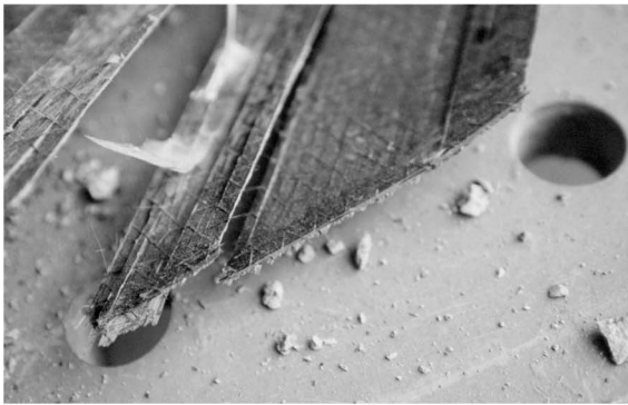
(a) Rupture of CFRP sheet on the tension side of Beam B3
