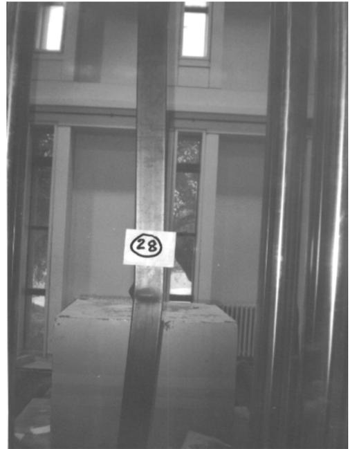
Fig. 3 Column C28-N filled with normal concrete after failure at midheight
