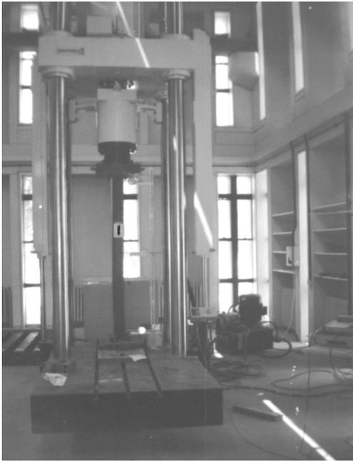
Fig. 2 Load application on column specimen
