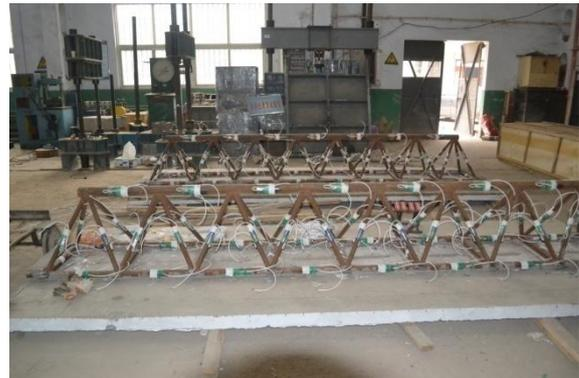
Fig. 4 SCCTB specimens
