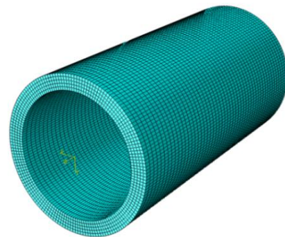
Fig. 2 Three dimensional mesh elements of the cylindrical shell
