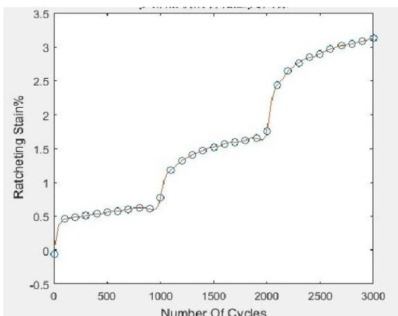
Fig. 13 The curve of ratcheting strain versus number of cycling with different mean stress and its history
