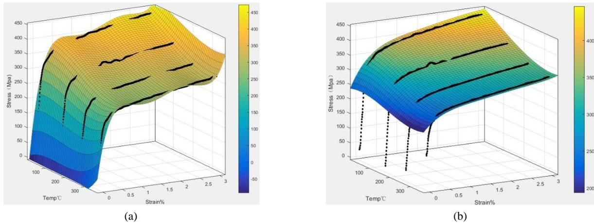
Fig. 9 Prediction results in three dimensions of uniaxial tension of Z2CND18.12N austenitic stainless steel at different temperatures based on neural network
