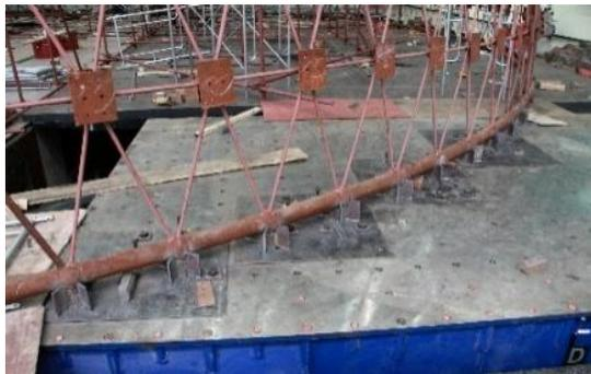
Fig. 3 Constraints on shaking table
