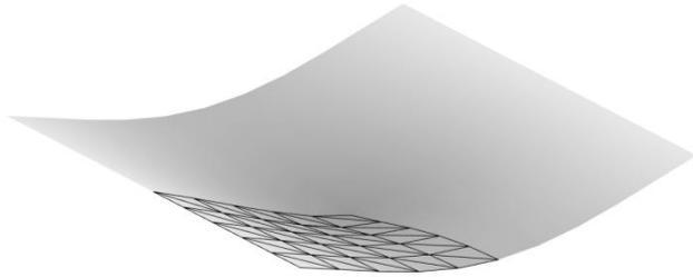
Fig. 4 Deformed configuration of shallow panel at the end of loading steps
