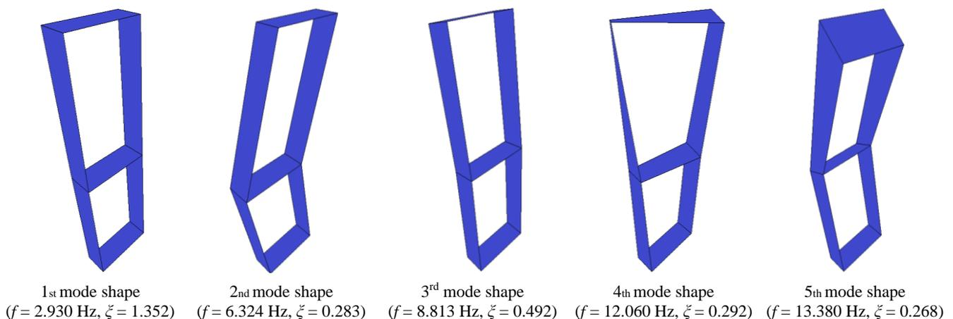
Fig. 9 Experimentally identified mode shapes of retrofitted model steel structure
