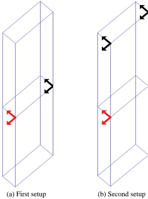
Fig. 3 Accelerometers location of experimental model in the 3D view
