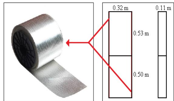
Fig. 7 GFRP composite and using details
