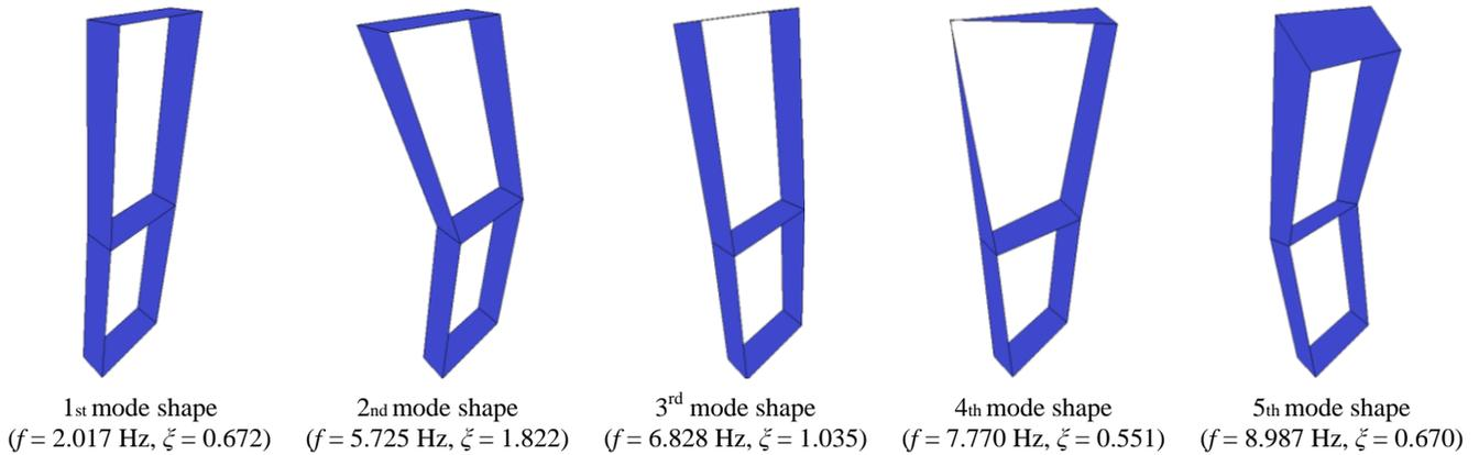
Fig. 6 Experimentally identified mode shapes of model steel structure
