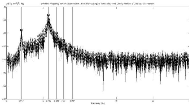
Fig. 5 Singular values of spectral density matrices (model steel structure)
