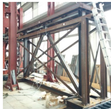
Fig. 4 Assembled EBF and setup of the test in the lab
