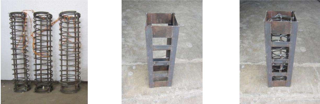
Fig. 3 Steel and reinforcing cages after construction
