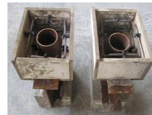
(b) Molding and rebar replacement
