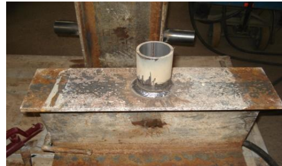
Fig. 2 Pipe shear connector-Vertical Pipe
