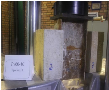
Fig. 6 Push-out test setup
