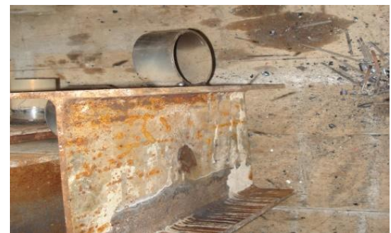
Fig. 3 Pipe shear connector-Horizontal Pipe
