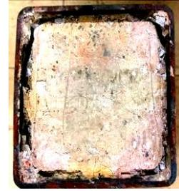
(b) Failure model of loading end
