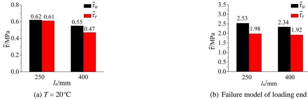
Fig. 14 Effect of anchorage length on bond strength
