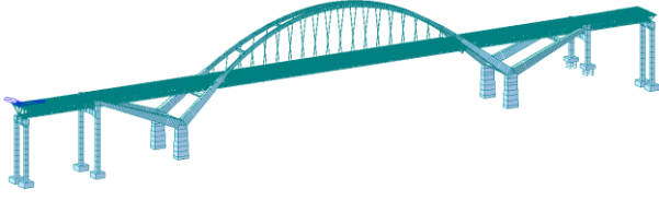
Fig. 10 Finite element model of the bridge
