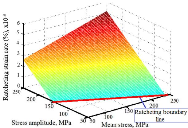
Fig. 9 Three dimensional ratcheting response surface
