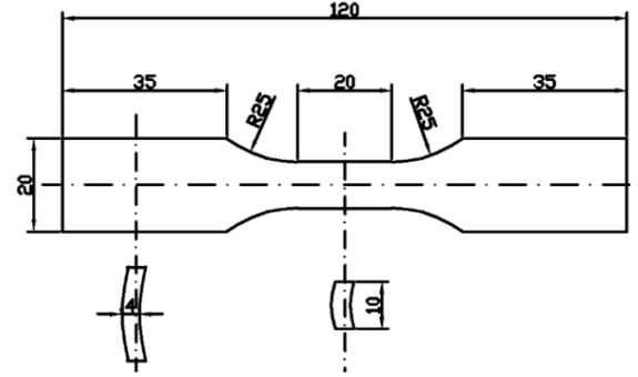
Fig. 2 Plate tension specimen
