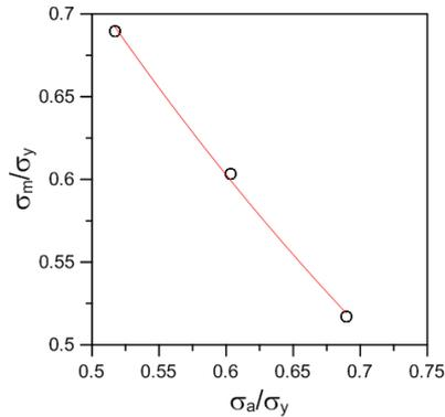
Fig. 8 Mean stress and stress amplitude relationship at yield stress of 290 MPa
