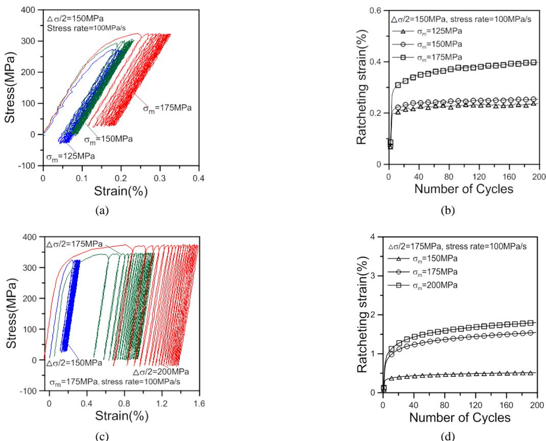
Fig. 4 Uniaxial ratcheting behavior with the constant amplitude of 150 MPa and 175 MPa under different mean stresses
