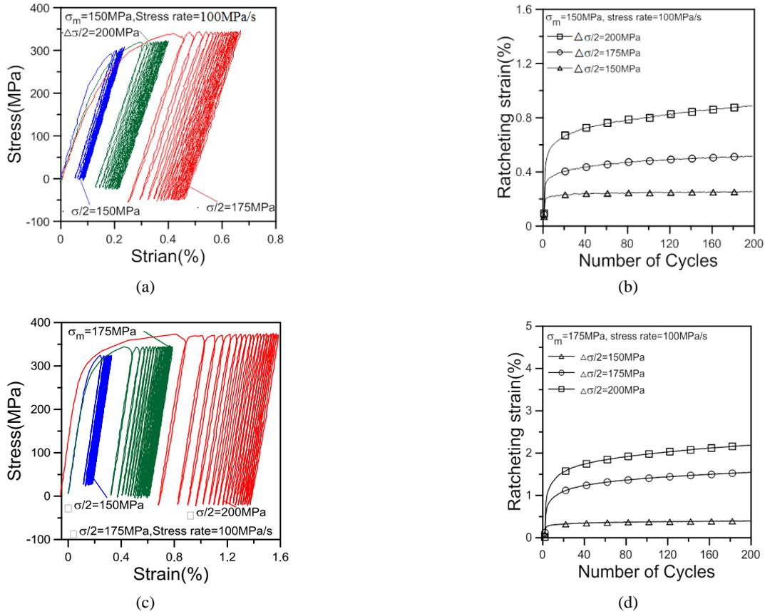
Fig. 5 Uniaxial ratcheting tests with the constant mean stress of 150 MPa and 175 MPa and different stress amplitudes
