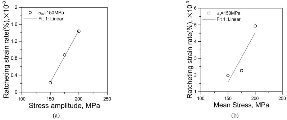
Fig. 7 (a) Ratcheting strain rate vs. stress amplitude at constant mean stress of 150 MPa; (b) Ratcheting strain rate vs. mean stress at constant stress amplitude of 150 MPa
