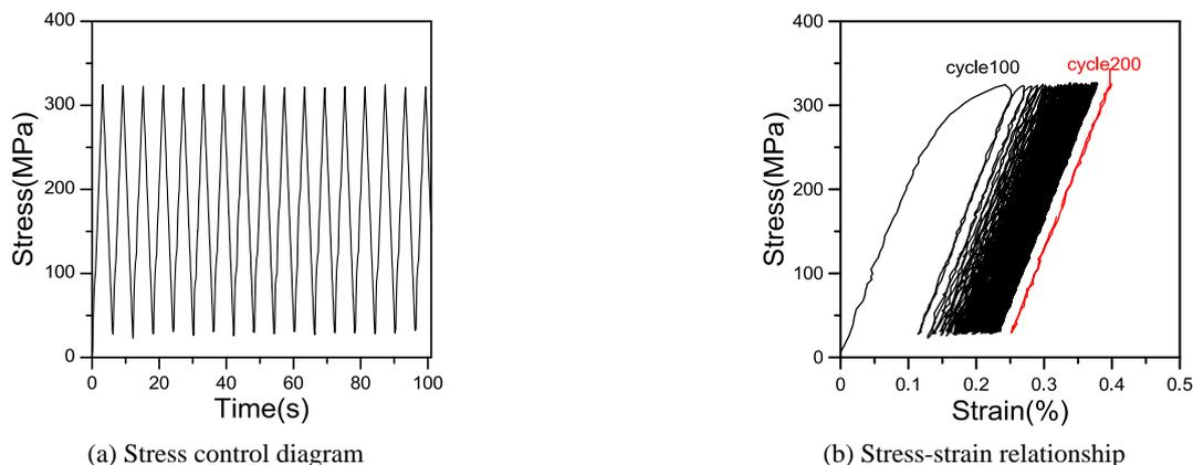
Fig. 2 Stress control and stress vs strain curve
