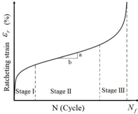
Fig. 1 Schematic triphasic trend of ratcheting strain over a stress cycles
