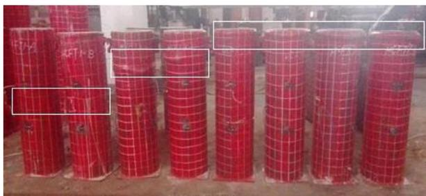
(a) Comparison of steel tube buckling
