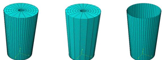
(a) Whole FE model (b) Concrete element (c) Steel element
