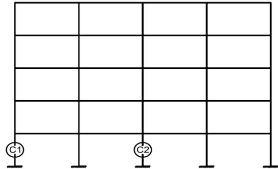
Fig. 2 Elevation of model and column removal cases
