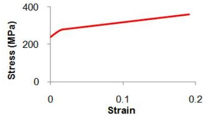
Fig. 5 plastic properties of steel materials
