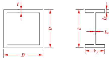
Fig. 6 Geometric dimensions of the frame sections
