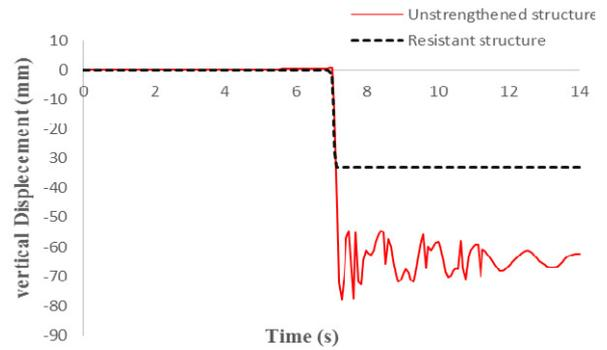
Fig. 10 Vertical displacement of the point at top of the removed middle column versus time
