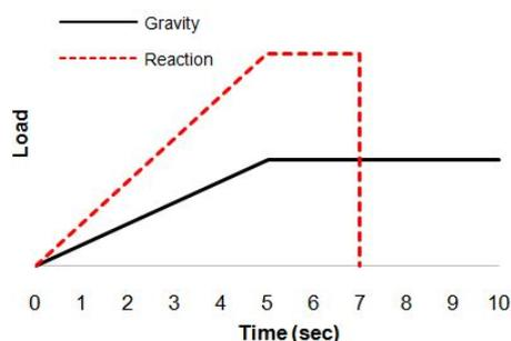
Fig. 1 Reaction approach, sudden column removal and linear increased gravity load
