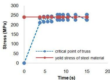
Fig. 9 Stress in critical part (which is shown in figure 6) of vierendeel frame
