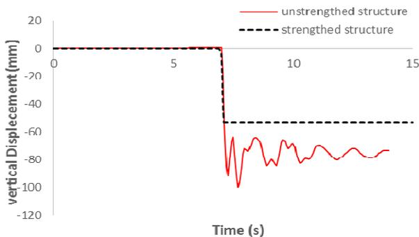
Fig. 8 Vertical displacement of the point at top of the removed exterior column versus time
