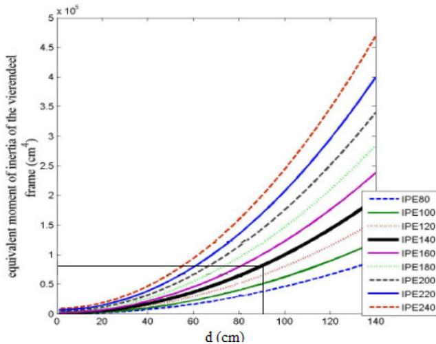
Fig. 14 Relationship between variable  $d$  and required equivalent moment of inertia of the vierendeel peripheral frame ( $I_{ve}$ ), for 9 types of rolled sections
