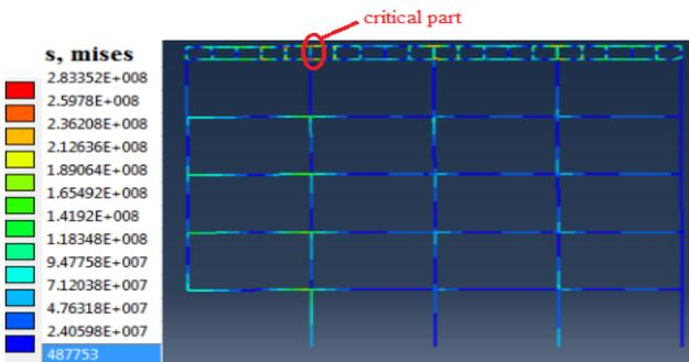
Fig. 7 Stress contour after column removal
