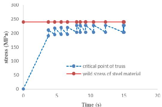
Fig. 11 Stress in critical part of vierendeel truss frame while middle column is removed
