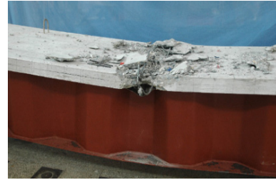
(e) Crushed concrete top slab
