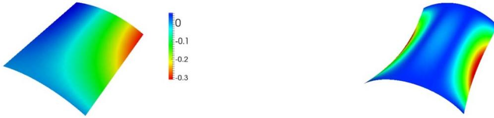
Fig. 7 Scordelis-Lo roof, vertical displacement at the midpoint of free edge
