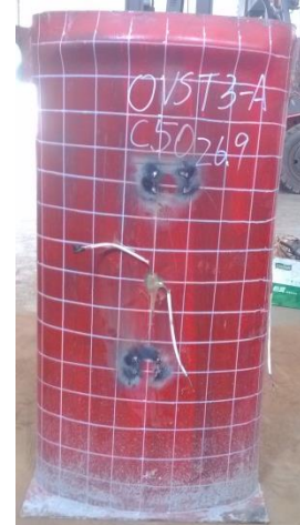
(b) E-CFT stub column
