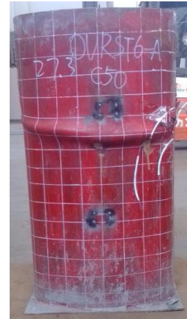
(a) RE-CFT stub column
