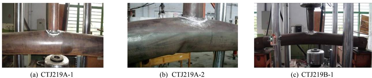
Fig. 16 Failure modes of the specimens in group CTJ219
