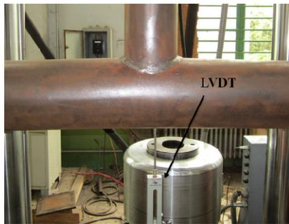
Fig. 10 LVDT at the bottom of the chord
