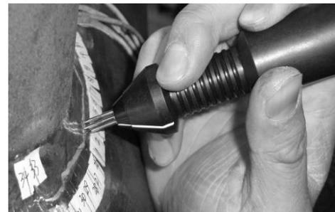
Fig. 8 Crack gauge for measuring crack depth and length
