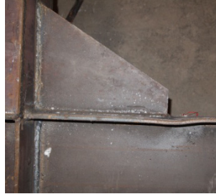
(e) Buckling occurred at beam end
