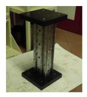
Fig. 5 Specimen ready for a stub-column testhpg
