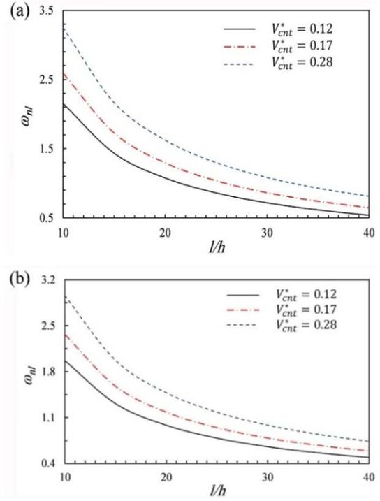
Fig. 5 Dimensionless nonlinear frequencies versus slenderness ratio for S-S CNTRC beams at  $a = 0.5$ : (a) UD; and (b) FG
