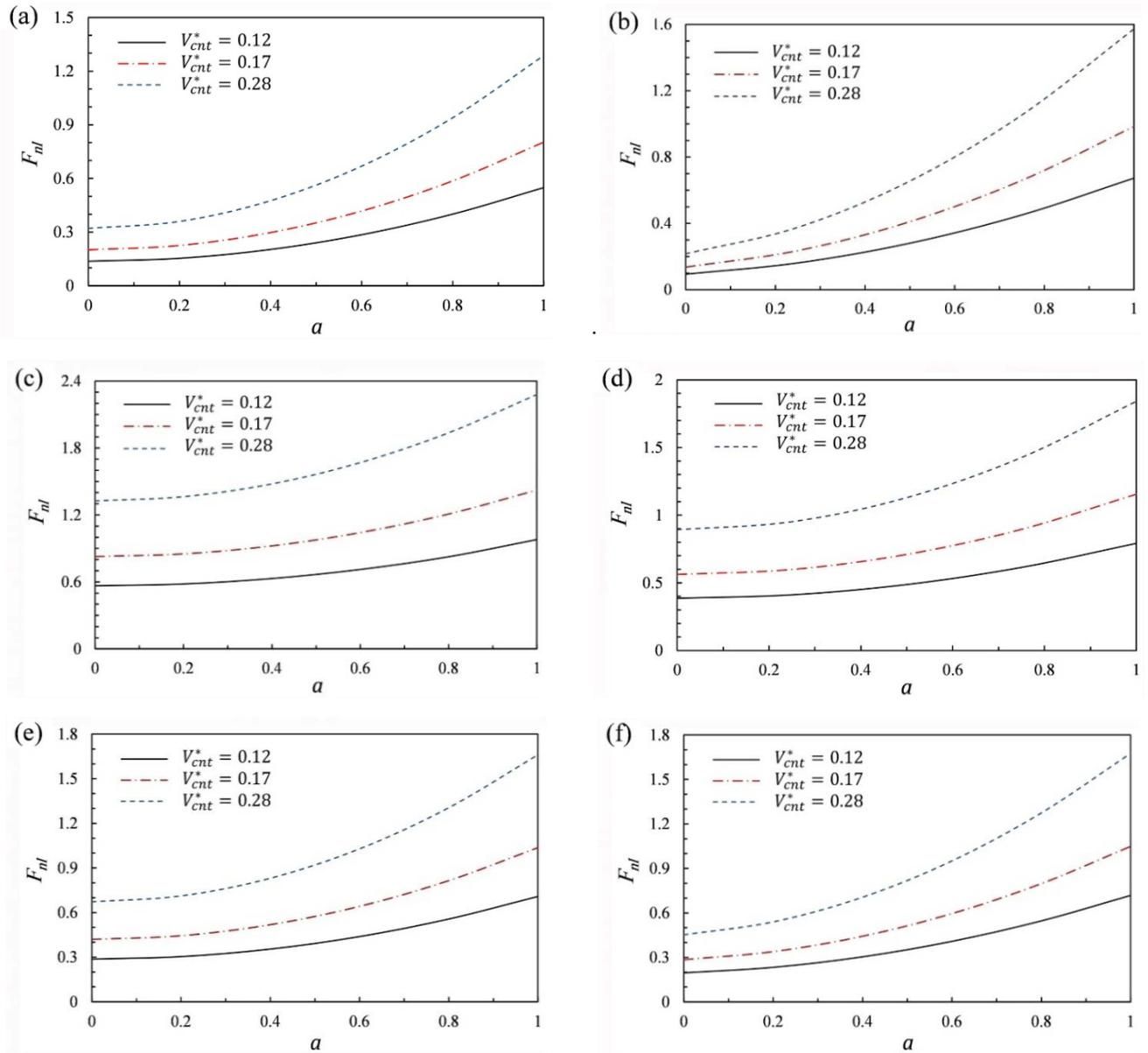
Fig. 7 Dimensionless post-buckling loads versus dimensionless maximum deflection of CNTRC beams with different volume fractions: (a) S-S UD; (b) S-S FG; (c) C-C UD; (d) C-C FG; (e) C-S UD; and (f) C-S FG
