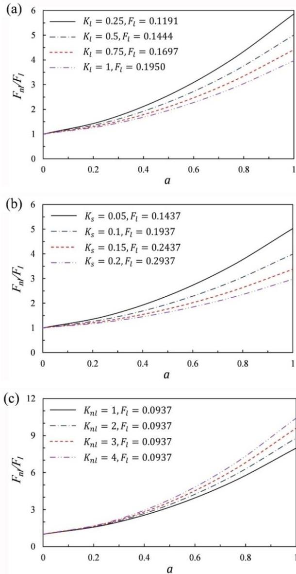
Fig. 9 Post-buckling load ratios versus dimensionless maximum deflection of S-S FG-CNTRC beams with  $V_{cnt}^* = 0.12$  for different values of foundation parameters: (a)  $K_l$  ( $K_s = K_{nl} = 0$ ); (b)  $K_s$  ( $K_l = K_{nl} = 0$ ); and (c)  $K_{nl}$  ( $K_l = K_s = 0$ )
