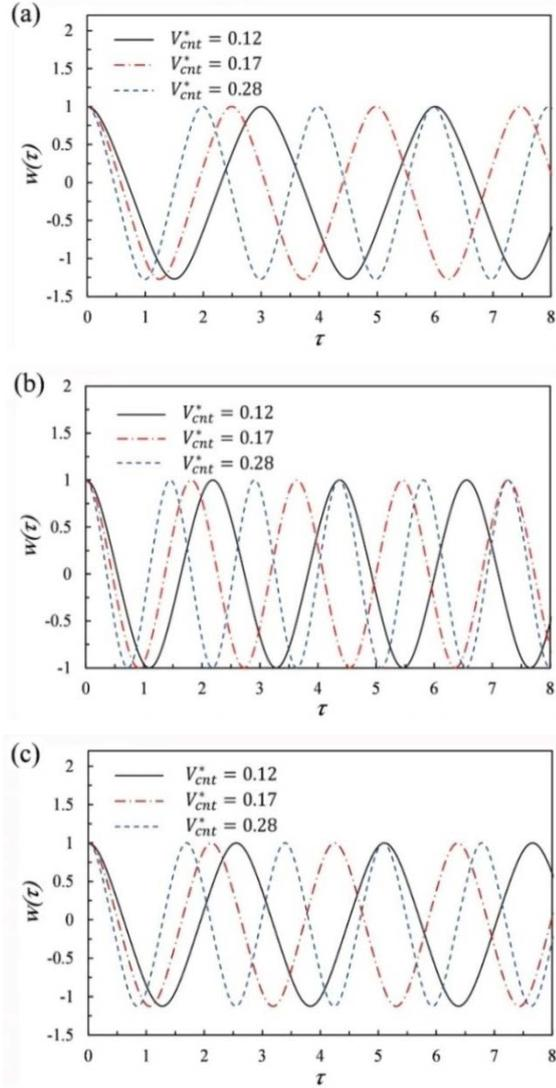
Fig. 4 Vibration response of FG-CNTRC beams at  $a = 1$ : (a) S-S; (b) C-C; and (c) C-S
