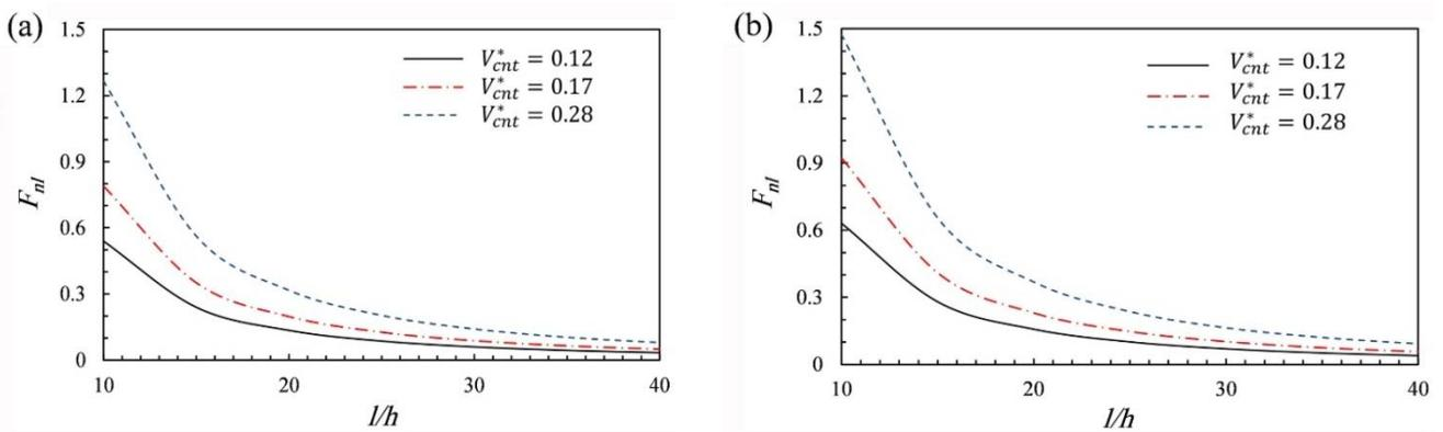
Fig. 8 Dimensionless post-buckling loads versus slenderness ratio for S-S CNTRC beams at  $a = 0.5$ : (a) UD; and (b) FG
