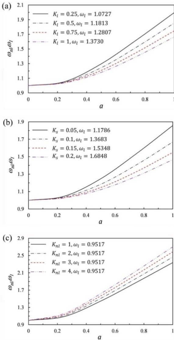
Fig. 6 Nonlinear frequency ratios versus vibration amplitude of S-S FG-CNTRC beams with  $V_{cnt}^* = 0.12$  for different values of foundation parameters: (a)  $K_I$  ( $K_S = K_{nl} = 0$ ); (b)  $K_S$  ( $K_I = K_{nl} = 0$ ); and (c)  $K_{nl}$  ( $K_I = K_S = 0$ )
