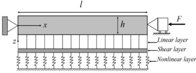
Fig. 2 Geometry of the FG-CNTRC beam on nonlinear elastic foundation
