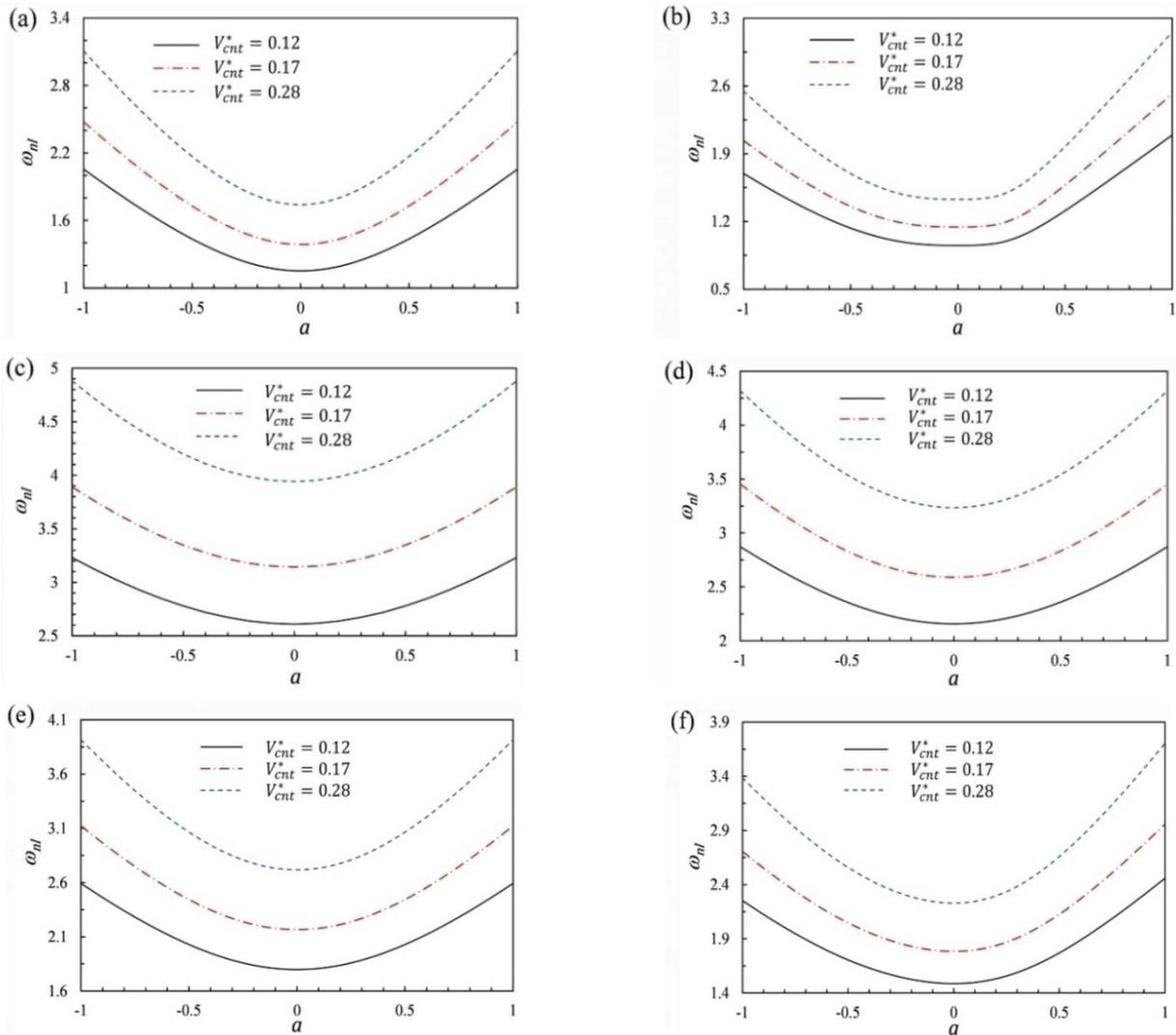
Fig. 3 Dimensionless nonlinear frequencies versus vibration amplitude for CNTRC beams with different volume fractions: (a) S-S UD; (b) S-S FG; (c) C-C UD; (d) C-C FG; (e) C-S UD; and (f) C-S FG
