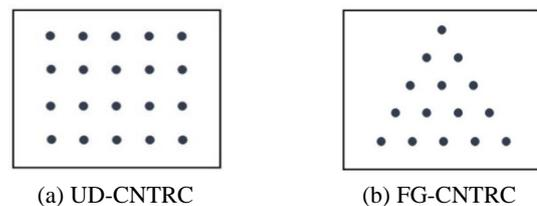
Fig. 1 SWCNTs distribution patterns in the FG-CNTRC beam
