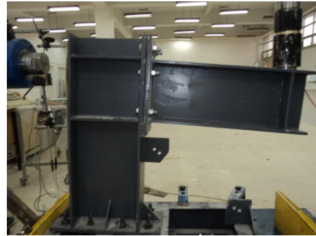
Fig. 9 Connection deformation for specimen C2
