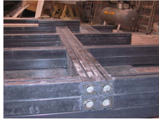
Fig. 3 Fabrication of the GFRP bridge deck, showing the configuration of the transverse beams
