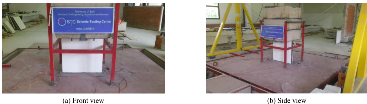
Fig. 2 Tested structure on the shake-table
