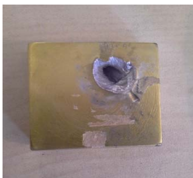
Fig. 9 14 mm thick 1040 steel after the shot
