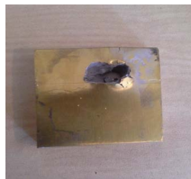
Fig. 8 9 mm thick titanium nitride coated 1040 steel after the shot
