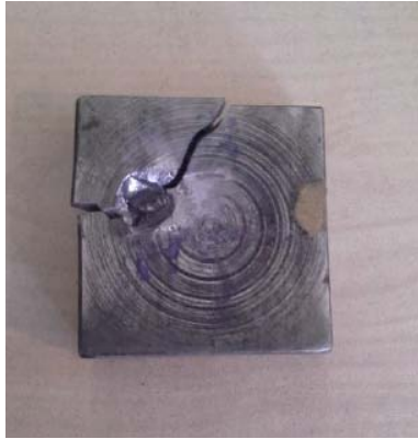
Fig. 9 14 mm thick 1040 steel after the shot
