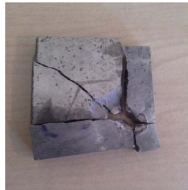
Fig. 7 9 mm thick 1040 steel after the shot
