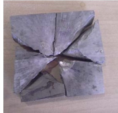
Fig. 11 9 mm thick 2842 steel after the shot
