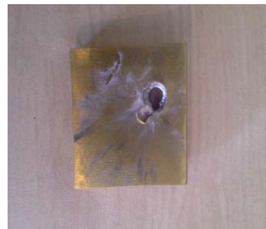
Fig. 7 9 mm thick 1040 steel after the shot
