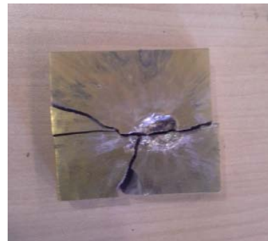
Fig. 12 9 mm thick titanium nitride coated 2842 steel after the shot
