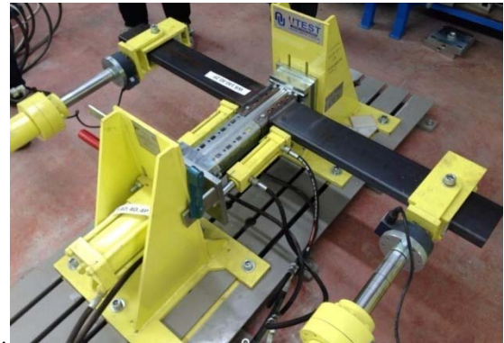
Fig. 3 Experimental setup for cyclic testing of rack beam-to-column connections
