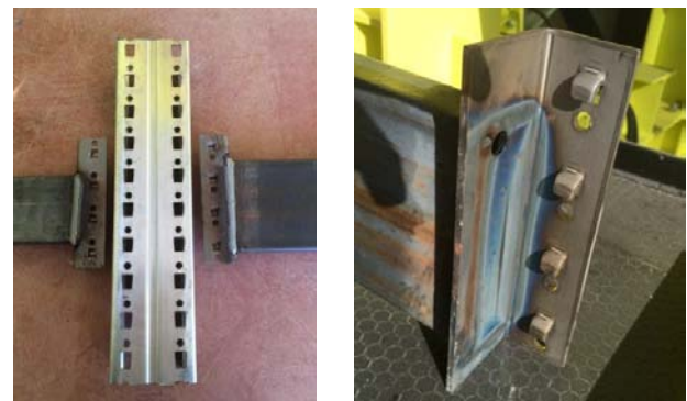
Fig. 1 Typical hooked beam-to-column connection in storage rack frames
