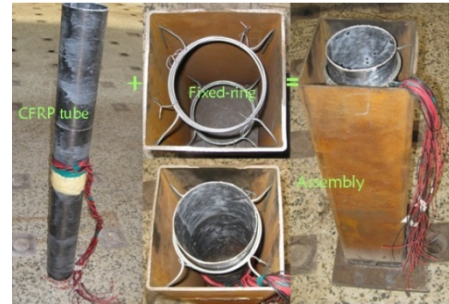
Fig. 3 Assembling of specimen
