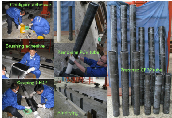
Fig. 2 Fabrication of CFRP tube
