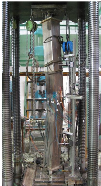
Fig. 11 Typical failure mode of medium long column
