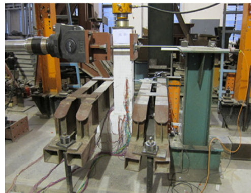
Fig. 2 Cyclic loading tests of SRRC columns
