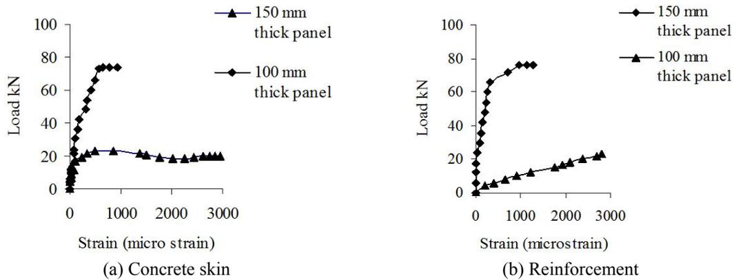
Fig. 3 Variation of load strain profile in concrete skin and reinforcement for different solidity ratios
