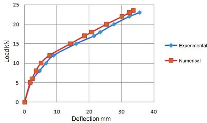
Fig. 10 Flexural load vs displacement (at centre) – 100 mm thick panels
