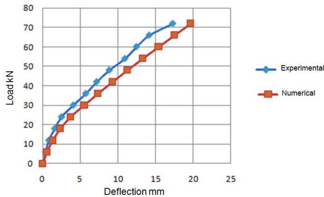
Fig. 13 Flexural load vs displacement (at load points) – 150 mm thick panels
