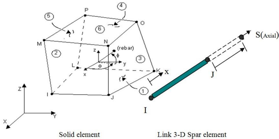
Fig. 6 FE elements used for modeling
