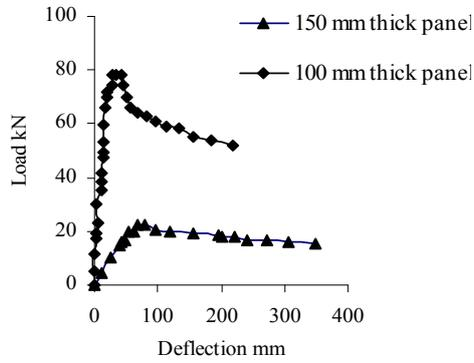
Fig. 2 Load deflection profile for different solidity ratios
