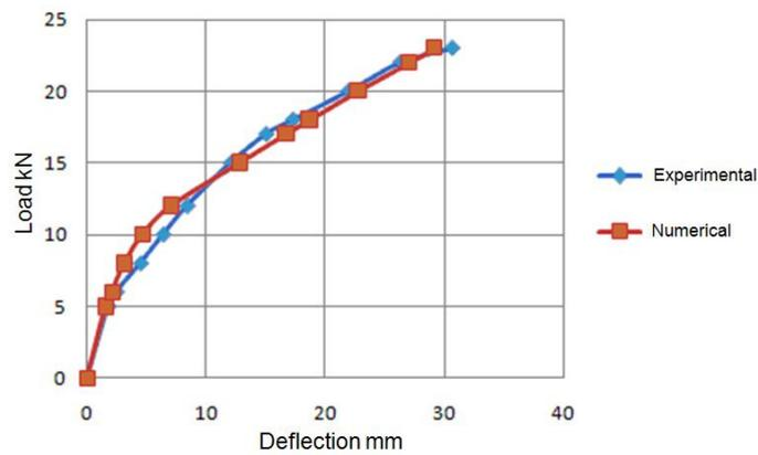
Fig. 11 Flexural load vs displacement (at load points) – 100 mm thick panels
