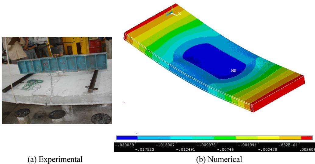
Fig. 8 Displacement contour of the panel under flexure
