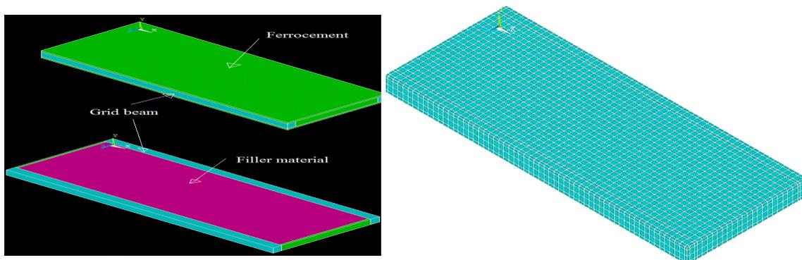
Fig. 5 Geometry and FE mesh of light weight concrete wall panel
