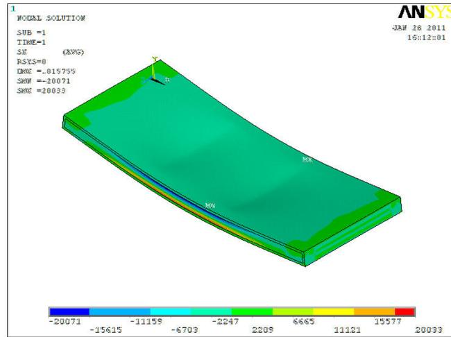
Fig. 9 Bending stress contour of the panel under flexure
