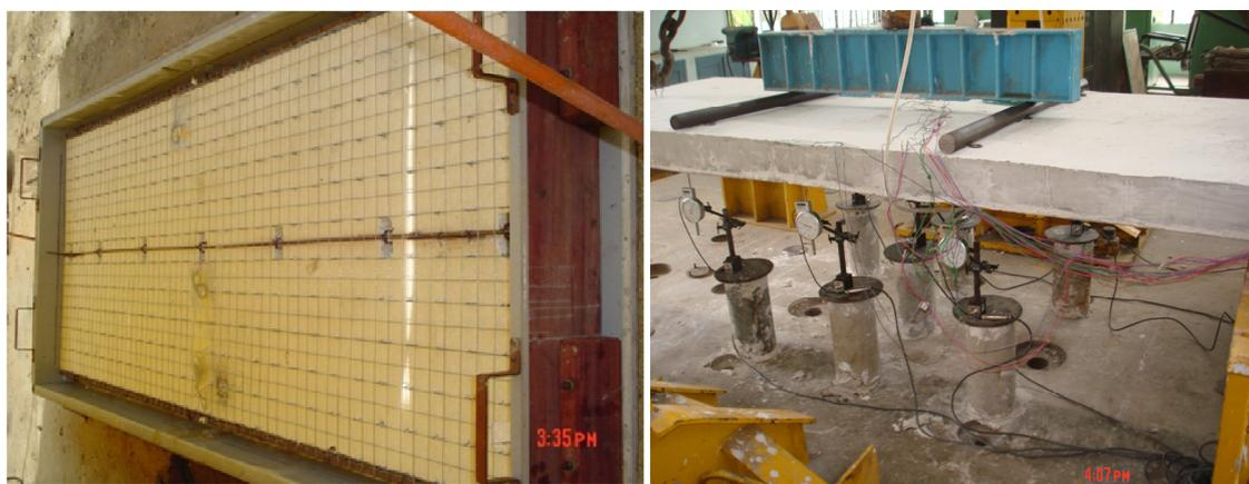
Fig. 1 Geometry of EPS inner Core with shear Connectors and test setup
