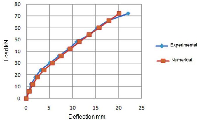
Fig. 12 Flexural load vs displacement (at centre) – 150 mm thick panels
