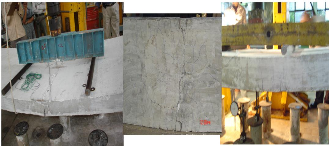
Fig. 4 Failure pattern of a wall panel under flexure
