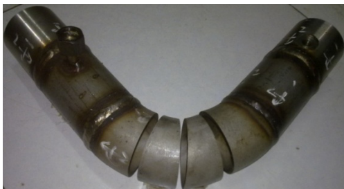
Fig. 14 Cut cross section of an elbow piping
