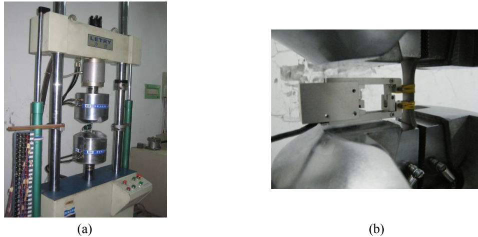
Fig. 2 Equipment: (a) Electro-hydraulic-servo fatigue testing machine; (b) Extensometer
