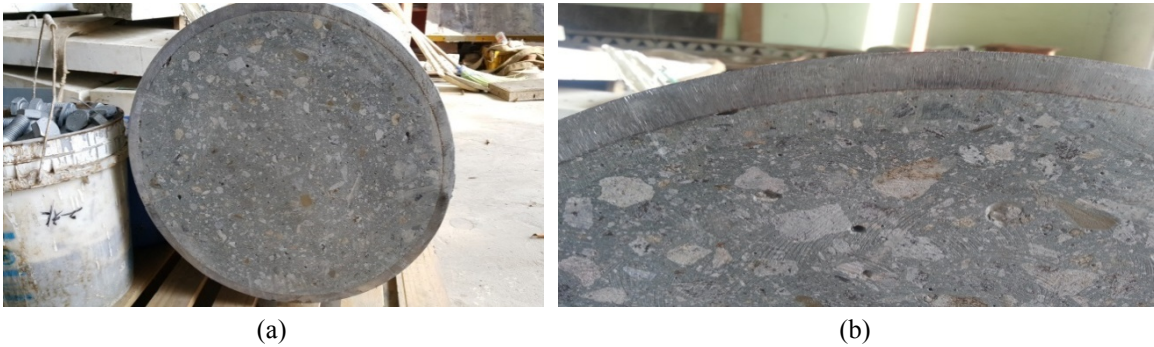
Fig. 18 Cutting section of CFT column (after test)
