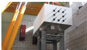
(h) Pier cap-column assembly
