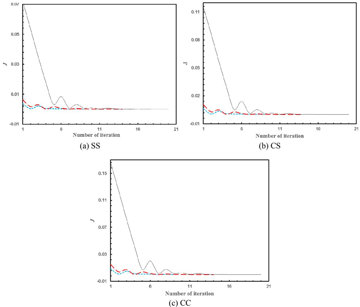
Fig. 3 Influence of start point on convergence and robustness of the conjugate gradient method for small scale parameter estimation of functionally graded nanobeams with different boundary conditions ( $\mu_{start}^2 = 4, n = 3, L/h = 20, \varepsilon = 10^{-6}$ )  $\mu_{start}^2 = 0$ : - - - - ;  $\mu_{start}^2 = 10$ : - · - · ;  $\mu_{start}^2 = 100$ : ———
