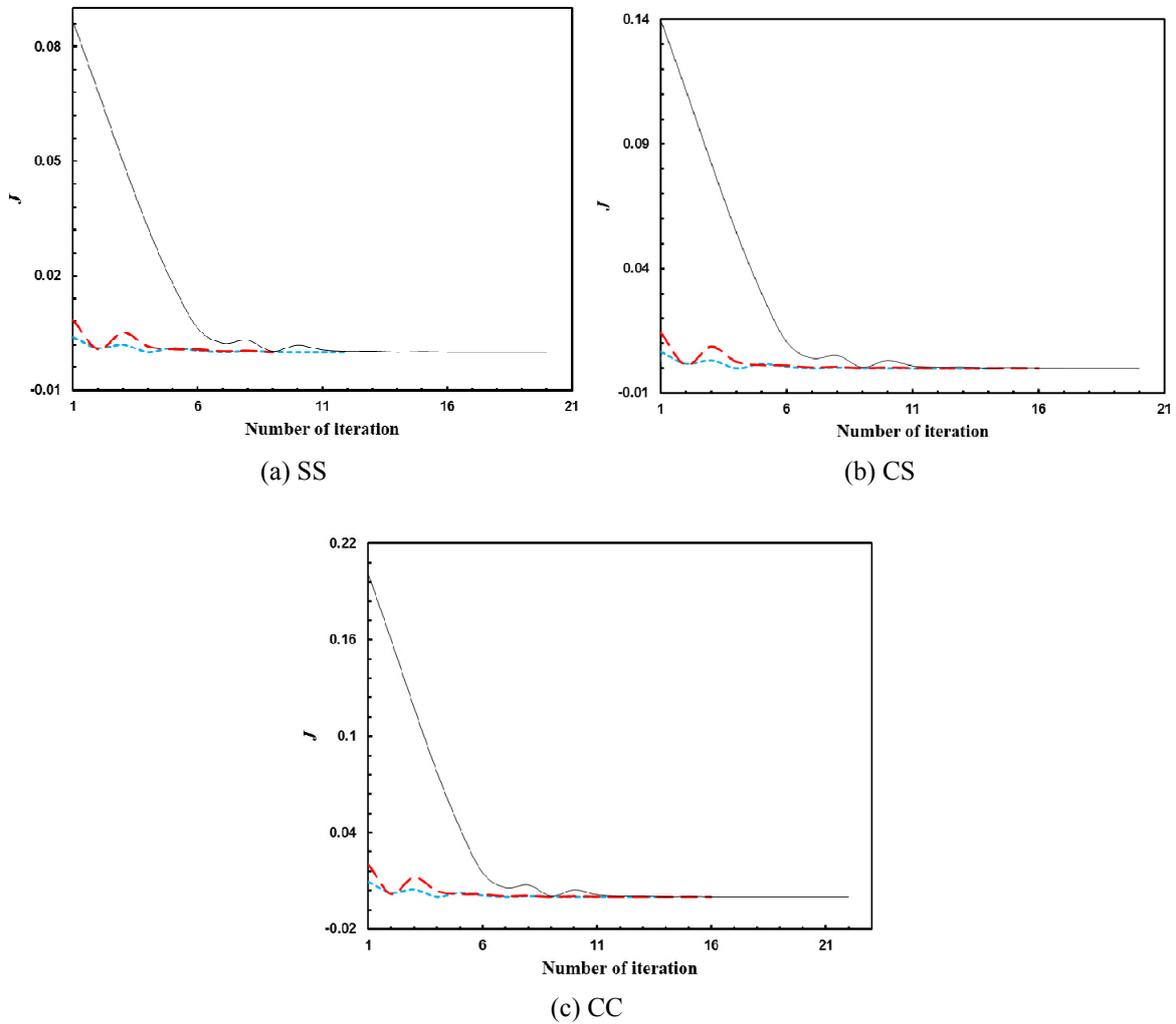
Fig. 2 Influence of start point on convergence and robustness of the conjugate gradient method for small scale parameter estimation of functionally graded nanobeams with different boundary conditions ( $\mu_{start}^2 = 2, n = 3, L/h = 20, \varepsilon = 10^{-6}$ )  $\mu_{start}^2 = 0$ : - - - - ;  $\mu_{start}^2 = 10$ : - · - · ;  $\mu_{start}^2 = 100$ : ———
