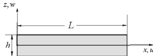
Fig. 1 The geometry of the nanobeam
