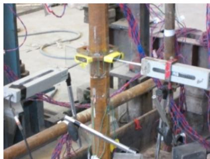
Fig. 4 Arrangement of displacement transducers
