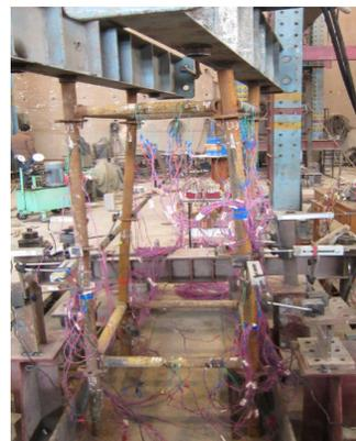
(b) Buckling mode of specimen 2
