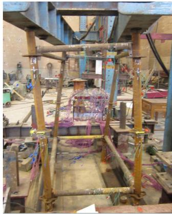
(c) Buckling mode of specimen 3
