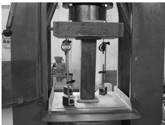
Fig. 3 Testing procedure of axially loaded columns
