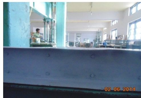
Fig. 11 Local buckling in the top flange
