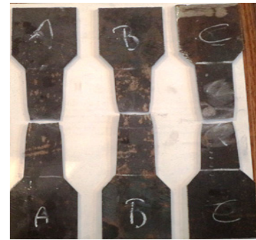
Fig. 7 Test specimens after tensile test
