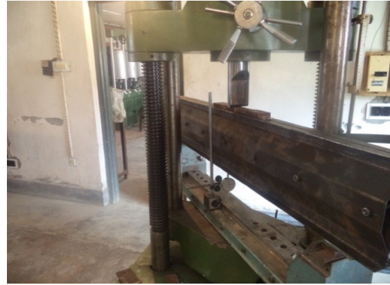
Fig. 9 Single point load arrangement
