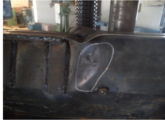
Fig. 13 Failure in the flange and web region
