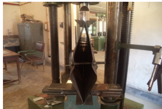
Fig. 15 Failure of sectional profile B by web buckling
