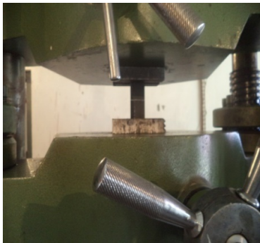
Fig. 5 Tensile test coupon in the U.T.M.
