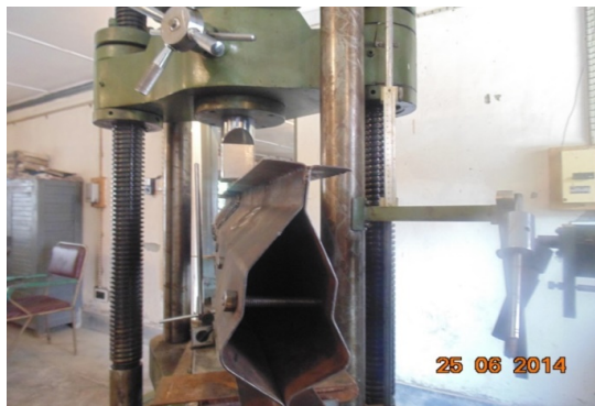
Fig. 14 Failure of sectional profile C by web buckling
