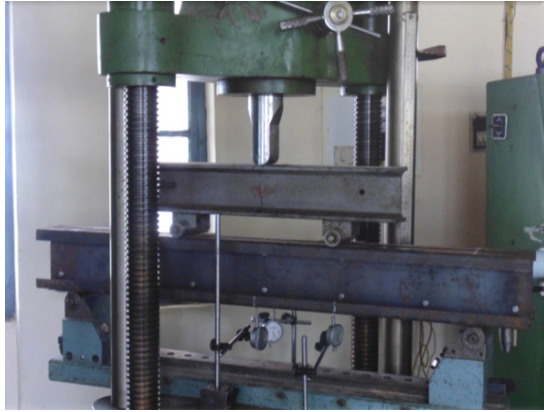
Fig. 8 Two point load arrangement
