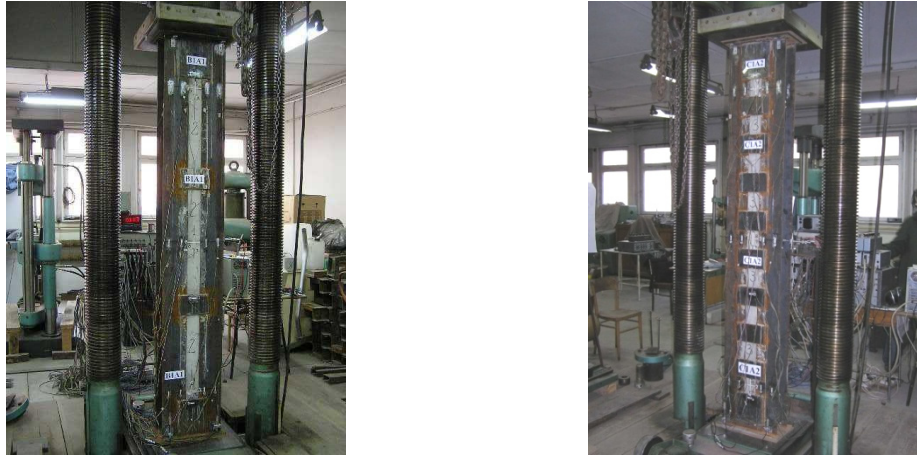
Fig. 7 A test stand for two-chord columns with batten spacing of: (a) 780 mm; (b) 240 mm
